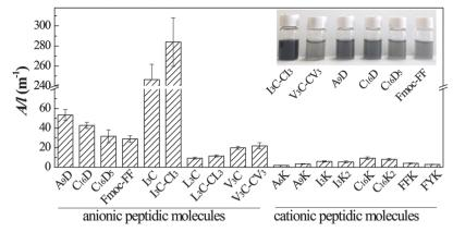
Fig. 2 The A/I values of the peptide-treated graphene dispersions that were obtained through centrifugation at 5000 rpm for 10 min after sonication in peptide solutions. The inset shows the photographs of several typical dispersions with relatively high exfoliation efficiency
