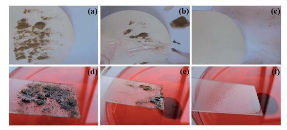
Self-cleaning properties of SiO<sub>2</sub>/PU in air (a-c) and contaminated by oil in air (d-f)
