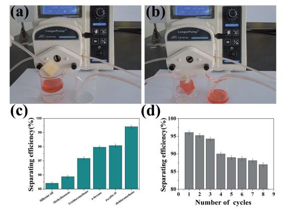
Fig. 8 (a and b) Photographs of the continuous absorption of silicone oil (dyed red) from water. (c) Oil/water separating efficiency. (d) Separating efficiency recyclability of the sponge.
