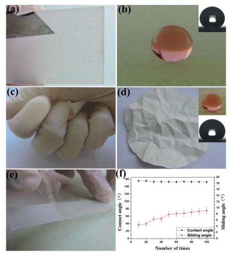
Fig. 4 Durability of the  $SiO_2/PU$  coating. (a) Scratched by a knife. (b) Photograph of a water droplet sitting on the coating surface after knife scratching (inset is the corresponding contact angle optical image). (c) Kneading tests of a coated filter paper. (d) Photograph of the filter paper after kneading tests (inset is the water droplet and contact angle optical image). (e) Tape peeling test. (f) Water contact angles and sliding angles after multiple cycles of tape peeling tests.
