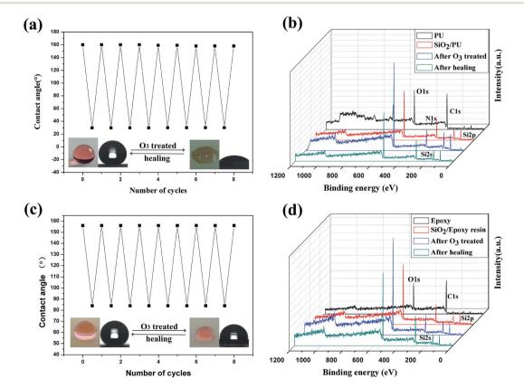
Fig. 6 Reversible superhydrophobic – hydrophilic transition of the as-prepared  $SiO_2/PU$  (a) and  $SiO_2/epoxy$  resin (c) under ozone irradiation and heat treatment. XPS analysis of  $SiO_2/PU$  coating (b) and  $SiO_2/epoxy$  resin (d) before and after ozone irradiation.
