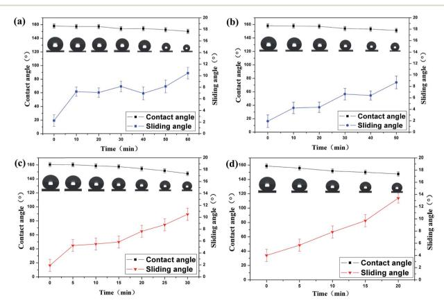
Fig. 5 Contact angles and sliding angles as a function of contact time with (a) acidic and (b) alkaline liquids on  $SiO_2/PU$  coatings, and (c) acidic and (d) alkaline on  $SiO_2/epoxy$  resin surfaces.
