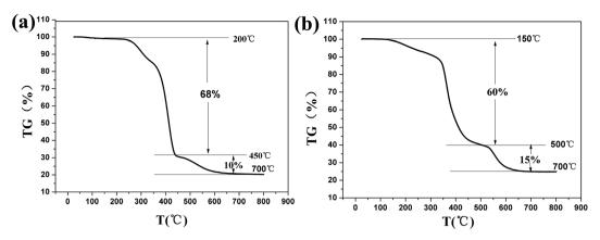
Fig. 3 TG images of (a) SiO<sub>2</sub>/PU and (b) SiO<sub>2</sub>/epoxy resin treated coatings
