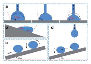
Fig. 3 Schematic illustrations of the technologies for characterization of the contact angle hysteresis: the advancing angle  $\Theta_{\mathsf{Adv}}$  and the receding angle  $\Theta_{\mathsf{Rec}}$  (a and b), sliding angle or rolling angle  $\Theta_{\mathsf{SA}}$
