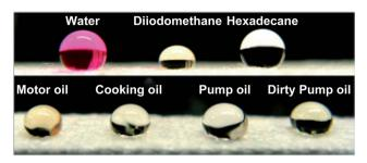
Fig. 6 Water droplet (dyed with rhodamine B) and various liquids on a cotton fabric grafted polymer with a concentration of 3 mg mL $^{-1}$ . (Reprinted from ref. 42 with permission).
