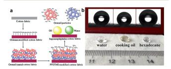
Fig. 5 (a) Schematic diagram of the fabrication process for superamphiphobic cotton fabrics. (b) Photographs of water, cooking oil and hexadecane droplets on the coated cotton fabrics. (Reprinted from ref. 38 with permission).
