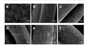
Fig. 8 SEM images of untreated cotton fabric (a and b) and cotton fabrics assembled with  $(PAH/SiO_2)_n$  multilayers: (c) n = 1, (d) n = 3, (e) n = 3= 5, and (f) n = 7. (Reprinted from ref. 54 with permission).
