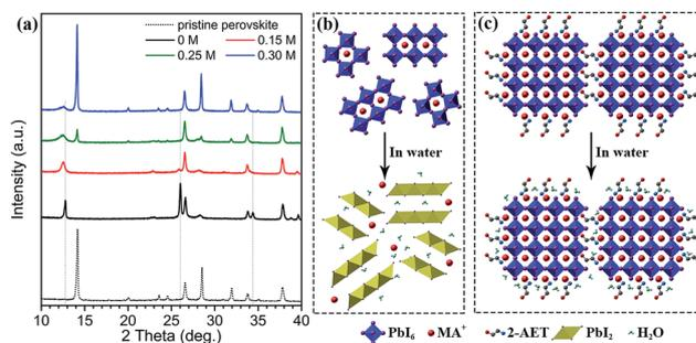
Fig. 7 XRD patterns (a) of  $\text{MAPbI}_3 \cdot (x)2\text{-AET}$  perovskite films immersed in water 15 s. Schematic diagram to show (b) the degradation process of  $\text{MAPbI}_3$  and (c) the mechanisms for water-resistant  $\text{MAPbI}_3 \cdot (x)2\text{-AET}$  perovskite in water.
