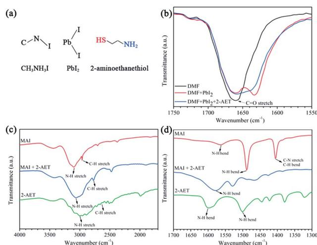
Fig. 1 Chemical structures (a) of MAI, PbI<sub>2</sub> and 2-AET; FTIR spectra of pure DMF, PbI<sub>2</sub> DMF solution and 2-AET/PbI<sub>2</sub> DMF solution in the range of 1750–1550 cm<sup>-1</sup> (b); FTIR spectra of MAI, 2-AET and MAI·2-AET solid complexes in the range of 4000–1700 cm<sup>-1</sup> (c) and 1700–1300 cm<sup>-1</sup> (d).
