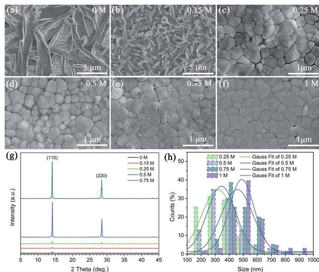
Fig. 2 SEM images of  $\text{MAPbI}_3\cdot(x)\text{2-AET}$  perovskite films prepared on FTO substrates, (a)  $x = 0$ ; (b)  $x = 0.15\text{ M}$ ; (c)  $x = 0.25\text{ M}$ ; (d)  $x = 0.5\text{ M}$ ; (e)  $x = 0.75\text{ M}$ ; (f)  $x = 1\text{ M}$ . XRD patterns (g) and statistical grain size distribution (h) of  $\text{MAPbI}_3\cdot(x)\text{2-AET}$  perovskite films.
