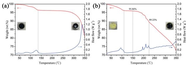
Fig. 8 DSC/TGA curves of MAPbI<sub>3</sub> (a) and MAPbI<sub>3</sub>·(0.75)2-AET (b) in the range of 30–350 °C at 5 °C min<sup>-1</sup> of heating rate. DSC curve (red line), TGA curve (blue line). The inset photographs are perovskite powders before (left) and after (right) measurement.
