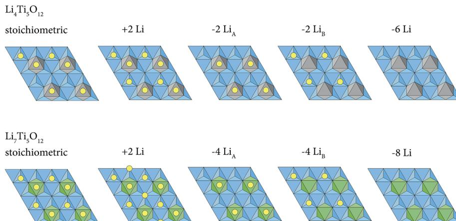
Fig. 6 Schematic of the stoichiometric and variable lithium-coverage A-terminated surface models that were calculated for  $\text{Li}_4\text{Ti}_5\text{O}_{12}$  and  $\text{Li}_7\text{Ti}_5\text{O}_{12}$ .
