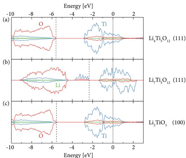
Fig. 8 Projected densities of states for the (a)  $\text{Li}_4\text{Ti}_5\text{O}_{12}$  (111), (b)  $\text{Li}_7\text{Ti}_5\text{O}_{12}$  (111), and (c)  $\alpha\text{-Li}_2\text{TiO}_3$  (100) surface slabs (13, 13, 12 layers). In each case the energy scale uses the vacuum energy as zero, shown with the solid vertical line. The energies of the highest occupied states are shown with dashed vertical lines. Contributions from Li s are shown in green, O p in red, and Ti d in blue.
