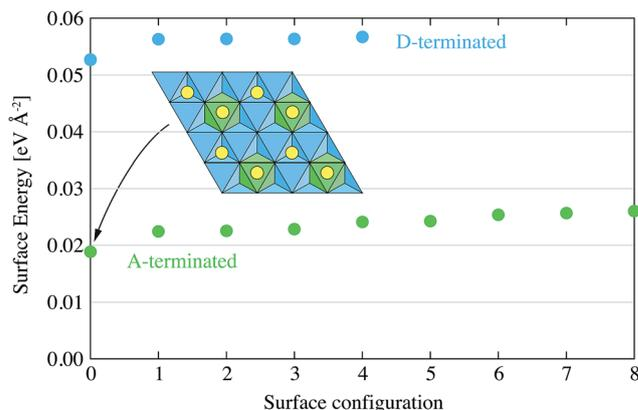
**Fig. 4** Surface energies in  $\text{eV } \text{\AA}^{-2}$  of the A-terminated and D-terminated  $\text{Li}_7\text{Ti}_5\text{O}_{12}$  (111) surface slabs. Blue and green octahedra show titanium and lithium occupied subsurface sites, respectively. Yellow circles show lithium positions.
