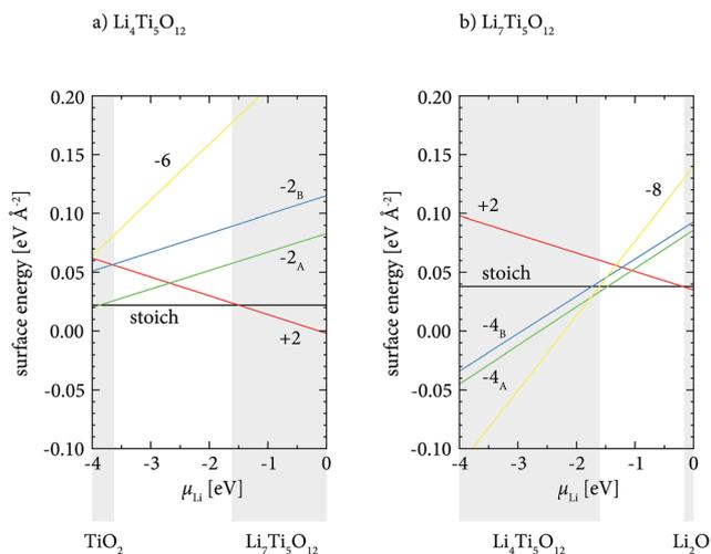
Fig. 7  $\mu_{\text{Li}}$ -Dependent surface energies for A-terminated  $\text{Li}_4\text{Ti}_5\text{O}_{12}$  and  $\text{Li}_7\text{Ti}_5\text{O}_{12}$  (111) surfaces. The shaded regions show lithium chemical potentials where  $\text{Li}_4\text{Ti}_5\text{O}_{12}$  and  $\text{Li}_7\text{Ti}_5\text{O}_{12}$  are predicted to be thermodynamically unstable for unconstrained oxygen/titanium chemical potentials.
