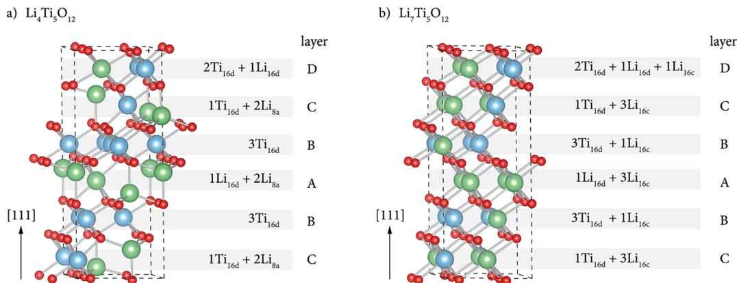
Fig. 2 Structures of (a)  $\text{Li}_4\text{Ti}_5\text{O}_{12}$ , and (b)  $\text{Li}_7\text{Ti}_5\text{O}_{12}$ , with the (111) close-packed direction oriented along  $c$ . For each close-packed layer, the relative number of Ti and Li cations in each crystallographic site are given. Both structures can be considered an array of (111) close-packed layers, with [...ABCDCBA...] stacking sequence.
