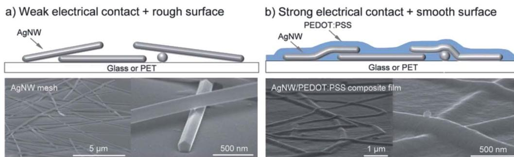
Fig. 2 (a) Bare AgNW mesh. (b) AgNW–PEDOT:PSS composite film (reproduced with permission. Copyright 2012, Royal Society of Chemistry).<sup>31</sup>
