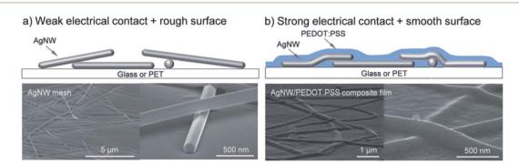
Fig. 2 (a) Bare AqNW mesh. (b) AqNW-PEDOT: PSS composite film (reproduced with permission. Copyright 2012, Royal Society of Chemistry). 31
