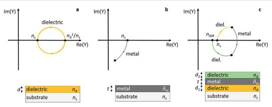
Fig. 10 Admittance plots for a dielectric layer (a), a metal layer (b), and a dielectric/metal/dielectric sandwich (c) on top of a substrate.
