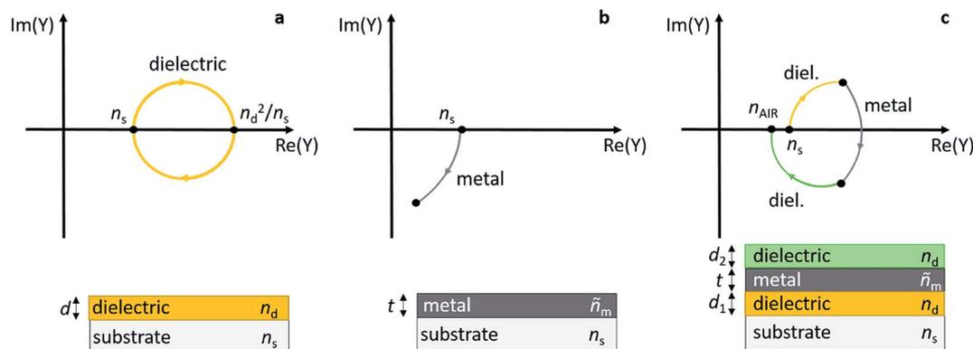
Fig. 10 Admittance plots for a dielectric layer (a), a metal layer (b), and a dielectric/metal/dielectric sandwich (c) on top of a substrate.
