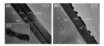
(a) Cross-sectional TEM image of the zinc-tin-oxide/Ag/zinctin-oxide (ZAZ) multilayer electrode. Inset: magnified view of the Ag layer in the sandwich. (b) Zinc-tin-oxide/Ag (ZA) structure deposited on a silicon substrate at room temperature, showing the agglomeration of an Ag layer after storage in ambient air for 500 h. Nominal thicknesses of the layers are 6 nm (Ag) and 60 nm (zinc-tin-oxide) (reproduced with permission. Copyright 2011, Elsevier). 192
