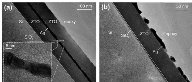
**Fig. 12** (a) Cross-sectional TEM image of the zinc-tin-oxide/Ag/zinc-tin-oxide (ZAZ) multilayer electrode. Inset: magnified view of the Ag layer in the sandwich. (b) Zinc-tin-oxide/Ag (ZA) structure deposited on a silicon substrate at room temperature, showing the agglomeration of an Ag layer after storage in ambient air for 500 h. Nominal thicknesses of the layers are 6 nm (Ag) and 60 nm (zinc-tin-oxide) (reproduced with permission. Copyright 2011, Elsevier).<sup>192</sup>
