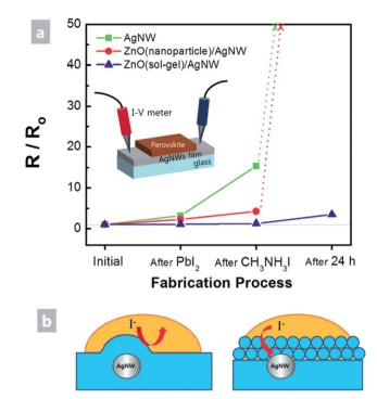
Fig. 7 (a) Resistance changes in AgNW films and ZnO/AgNW films during sequential perovskite deposition. After 24 h of aging, resistances were re-measured. (b) Schematics showing cross-sections of composite electrodes when the perovskite precursor solution containing iodine ions was coated on either the AgNW-sol-gel-derived (left) dense composite electrode or the AgNW-nano-particulate porous (right) composite electrode (reproduced with permission. Copyright 2016, Royal Society of Chemistry). 116
