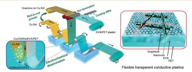
Fig. 3 Schematic of a R2R fabrication process for large-scale transparent electrodes of AgNWs and a hot-laminated graphene monolayer (reproduced with permission. Copyright 2015, American Chemical Society).<sup>57</sup>
