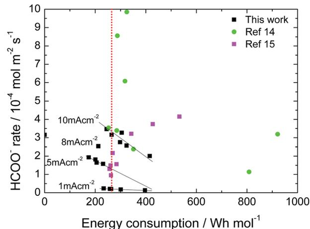
Fig. 8 Energy consumption of CO<sub>2</sub>R to formate using Sn-GDE in a filter-press EC cell at different production rates. Data from this work and ref. 14 and 15.
