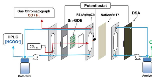
Fig. 1 Scheme of the electrochemical flow cell.
