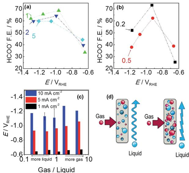
Fig. 7 Faradaic efficiency of formate versus Sn-GDE electrode potential: (a) gas/liquid = 1, 2 or 5 and (b) gas/liquid = 0.2 or 0.5 in 0.5 M NaHCO<sub>3</sub> for 200 C electrolysis. (c) CO<sub>2</sub> gas to 0.5 M NaHCO<sub>3</sub> electrolyte flow ratio effect on Sn-GDE electrode potential. (d) Schematic of gas and liquid flow over Sn-GDE, at G/L = 0.2 and 0.5 and G/L = 1, 2 and 5, left and right parts respectively.
