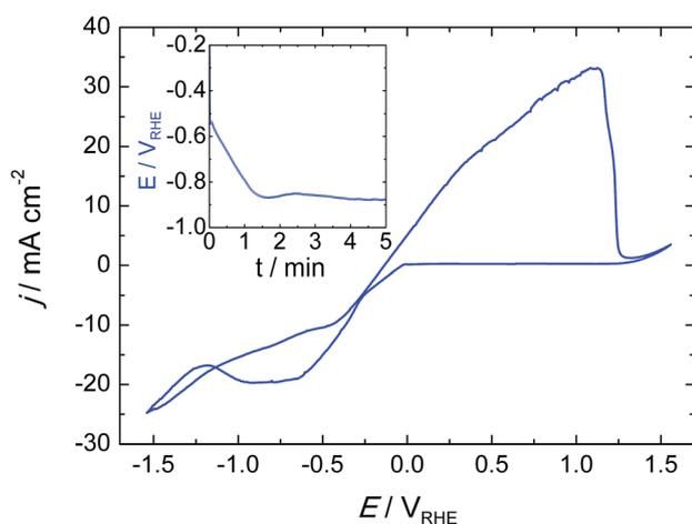
Fig. 2 Cyclic voltammogram for tin deposition and stripping on the gas diffusion electrode (C-Toray TGP-H-60) in pyrophosphate bath (pH 8.3) at a scan rate of  $20 \text{ mV s}^{-1}$ . Inset, chronopotentiometry at  $15 \text{ mA cm}^{-2}$  during Sn catalyst deposition.
