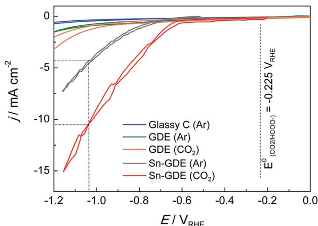
Fig. 4 Cyclic voltammogram on glassy carbon (GC), GDE and Sn-GDE under 10  $\text{mL min}^{-1}$  Ar or  $\text{CO}_2$  gas flow at a scan rate 20  $\text{mV s}^{-1}$  in 0.5 M  $\text{NaHCO}_3$  electrolyte (GC electrode was tested in a 3-electrode EC cell with  $\text{CO}_2$  bubbling while the other electrodes were in filter-press EC cells).
