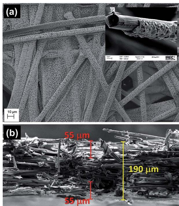
Fig. 3 (a) FE-SEM top view image of the Sn-GDE electrode obtained by electrodeposition of Sn at  $15 \text{ mA cm}^{-2}$  for  $4.5 \text{ C cm}^{-2}$  on C-Toray paper from pyrophosphate solution. Inset shows the Sn deposit on a carbon fiber. (b) FE-SEM cross-section of Sn-GDE.
