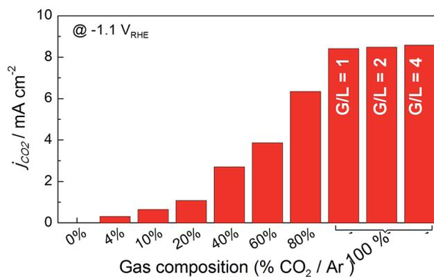
Fig. 6 Histogram of net current density for  $\text{CO}_2$  reduction on Sn-GDE obtained by subtracting the current density value of Ar from  $\text{CO}_2$  at  $-1.1 V_{\text{RHE}}$  in the CV scans (Fig. S5†). Data recorded in the filter-press cell in 0.5 M  $\text{NaHCO}_3$  ( $50 \text{ mL min}^{-1}$ ) by increasing the amount of gas by  $\text{CO}_2$  percentage in Ar gas flow (total flow  $50 \text{ mL min}^{-1}$ ). For G/L 2 and 4, 100 and 200  $\text{mL min}^{-1}$  of gas flow was used.
