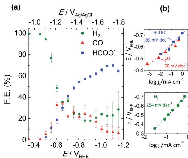
Fig. 5 (a) Total faradaic efficiency of  $\text{CO}_2$  reduction products at the end of 200 C of charge passed from the external circuit and (b) the corresponding Tafel plots for production of  $\text{HCOO}^-$ , CO and  $\text{H}_2$ .
