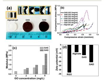
Fig. 4 (a) Photograph of alginate, GAS and GAD hydrogels for the mechanical property test, (b) compressive stress–strain profile and (c) Young's modulus of hydrogels at different GO concentrations, (d) zeta potential of RGO, alginate gel, GAS and GAD (GO concentration 8 mg mL $^{-1}$ ) at pH 8.
