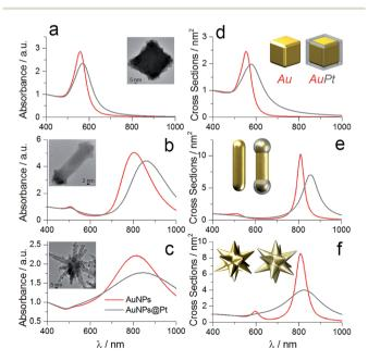
Fig. 2 Optical characterisation of the nanoparticles in solution. (a-c) Experimental and (d-f) simulated spectra of the bare gold (red) and Ptcoated (grey) nanoparticles with cubic (a, d), rod-like (b, e) and star-like morphology (c, f). Insets in (d-f) represent three-dimensional images of the particles used in simulations.
