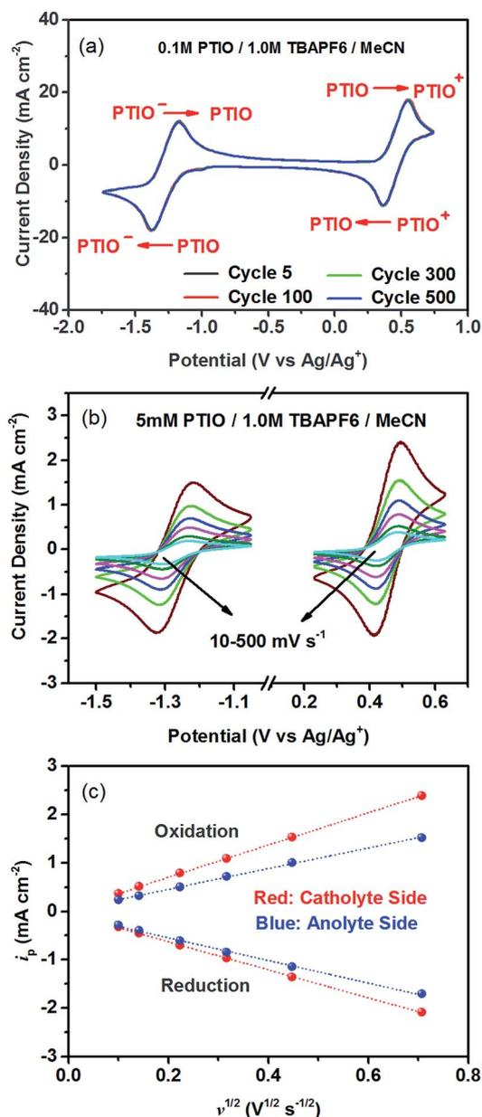
Fig. 1 CV curves of PTIO in a supporting electrolyte of 1.0 M TBAPF<sub>6</sub>/MeCN: (a) 500 cycles of repeated CV scans with 0.1 M PTIO at 100 mV s<sup>-1</sup>; (b) at different potential sweeping rates ( $\nu = 10, 20, 50, 100, 200$  and  $500$  mV s<sup>-1</sup>) with 5.0 mM PTIO; (c) linear relationship between  $i_p$  and  $\nu^{1/2}$  obtained from Randles–Sevcik analysis.
