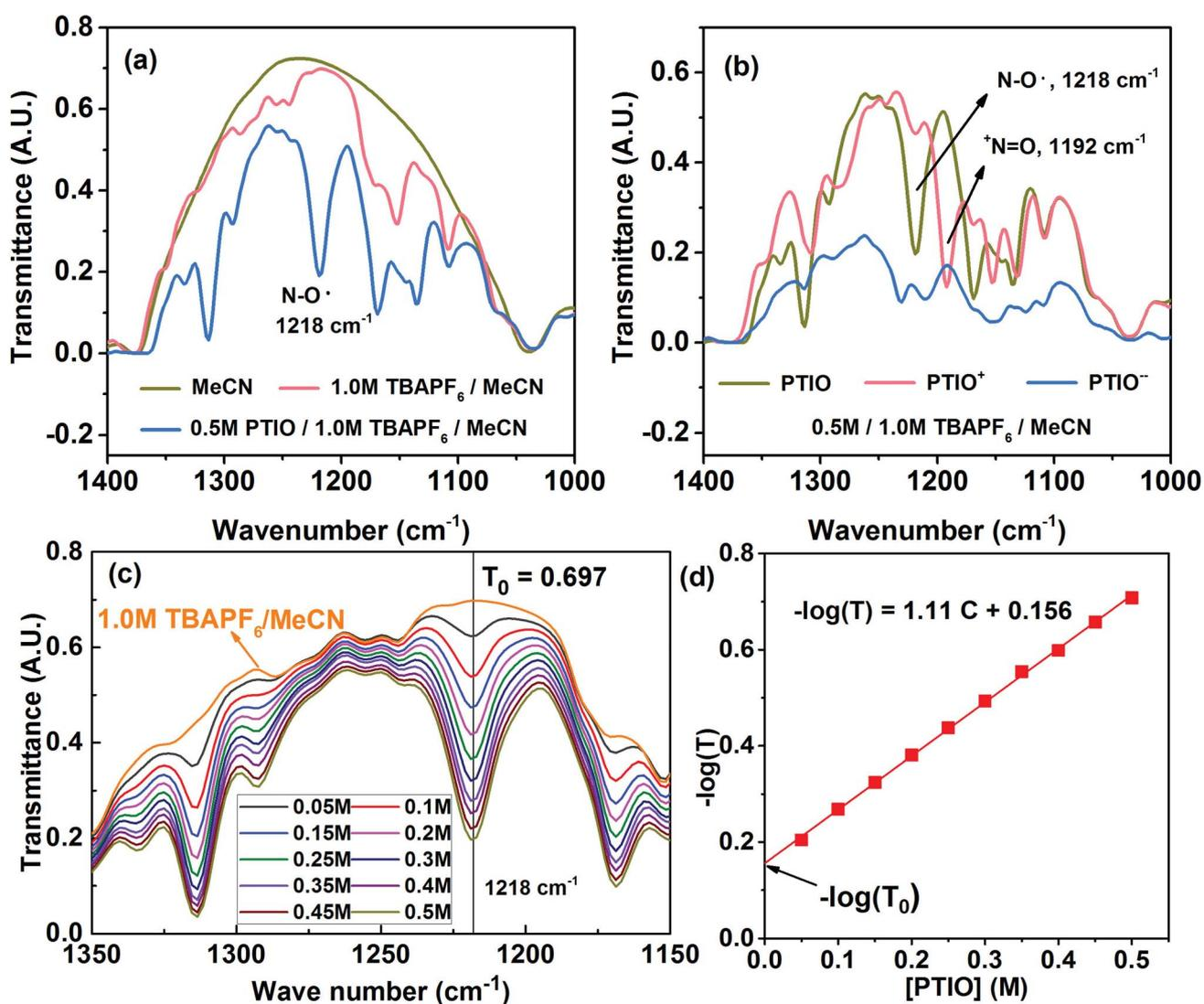
Fig. 4 FTIR of the PTIO species in the TBAPF<sub>6</sub>/MeCN electrolyte systems: (a) expanded spectral view for MeCN, 1.0 M TBAPF<sub>6</sub>/MeCN, and 0.5 M PTIO in 1.0 M TBAPF<sub>6</sub>/MeCN; (b) expanded spectral view of 0.5 M PTIO, PTIO<sup>+</sup>, and PTIO<sup>-</sup>; (c) expanded spectral view of PTIO in 1.0 M TBAPF<sub>6</sub>/MeCN with [PTIO] ranging from 0.05 M to 0.5 M; (d) derived linear  $-\log(T)$  vs. [PTIO] calibration curve based on the peak at 1218  $\text{cm}^{-1}$ .
