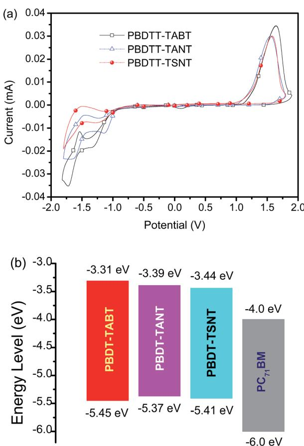
Fig. 4 (a) Cyclic voltammograms of the copolymer films. (b) HOMO and LUMO energy levels of the copolymers and PC<sub>71</sub>BM.
