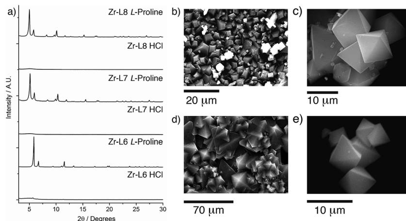
Fig. 2 (a) PXRD patterns showing the effects of incorporation of 5 equivalents of L-proline and one of HCl into solvothermal syntheses of Zr MOFs of **L6–L8** compared to addition of HCl alone. SEM images of the MOFs formed using this protocol: (b) **Zr-L5**, (c) **Zr-L6**, (d) **Zr-L7**, (e) **Zr-L8**.
