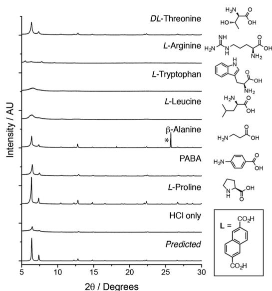
Fig. 1 Stacked PXRD patterns of **Zr–L5** synthesised with different amino acid modulators (five equivalents), compared with **Zr–L5** synthesised with one equivalent of HCl only and the pattern predicted from the previously reported crystal structure.<sup>9b</sup> An unknown crystal-line impurity, marked by an asterisk, was occasionally found in  $\beta$ -alanine modulated samples.
