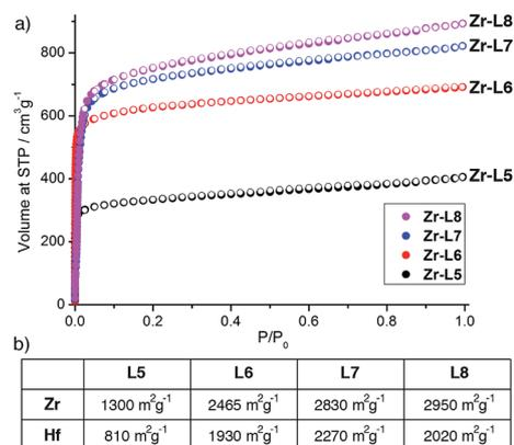
Fig. 6 (a) N<sub>2</sub> adsorption isotherms (77 K) for Zr-L5, Zr-L6, Zr-L7 and Zr-L8. (b) BET surface areas for all Zr and Hf MOFs, as derived from their N<sub>2</sub> adsorption isotherms.
