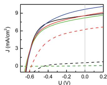
Fig. 1  $J$ - $V$  curves of pristine P3HT:PCBM solar cells (solid lines) and post-treated P3HT:PCBM solar cells (dashed lines) processed using chlorobenzene (black), toluene (blue), xylene (green) and dichlorobenzene (red), respectively.
