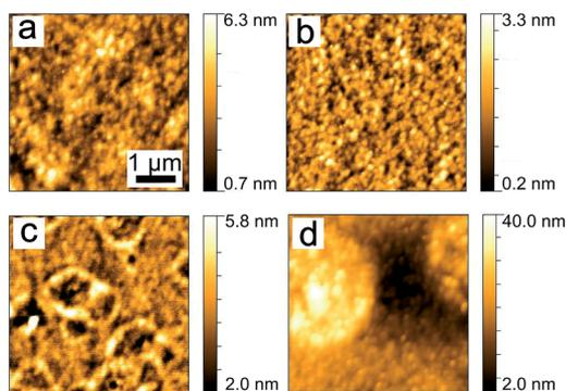
Fig. 3 AFM images ( $4 \times 4$ )  $\mu\text{m}^2$  of P3HT:PCBM films, post-treated with chlorobenzene (a), toluene (b), xylene (c) and dichlorobenzene (d) vapors. The corresponding rms roughness values are 8.6 Å, 4.7 Å, 7.8 Å and 79.8 Å, respectively.
