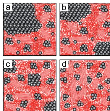
**Fig. 10** Schematic morphology of P3HT:PCBM films post-treated with chlorobenzene (a), toluene (b), xylene (c) and dichlorobenzene (d) vapors. The grey spheres correspond to PCBM, red tangled lines represent amorphous P3HT and red parallel lines are related to P3HT crystallites.
