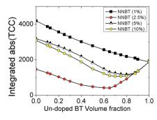
Fig. 5 The integrated absolute TCC response versus  $V_f$  of undoped BT for NNBT-BT ceramics based on Fig. 1. This provides a new method to identify the best combination of doped materials with undoped BT to minimise TCC in MLCCs.
