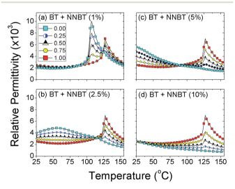
Fig. 3 Simulated permittivity-temperature profiles. These are FEM generated simulations of experimental input data for an undoped BT core surrounded by a shell phase of (a) 1%, (b) 2.5%, (c) 5% and (d) 10% doped NNBT. In each figure, different shell  $V_f$  values are plotted, i.e.  $V_f$ = 0.0 (all shell, xNNBT), 0.25, 0.50, 0.75 and 1.0 (all core, un-doped BT).
