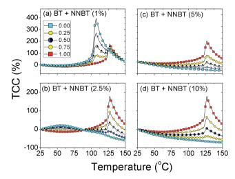
Fig. 4 Calculated TCC values versus temperature based on conversion of simulated  $\varepsilon_r$  to TCC values. Similar to Fig. 3, they are simulations of a BT core surrounded by a shell phase of (a) 1%, (b) 2.5%, (c) 5% and (d) 10% doped NNBT. In each figure, different shell  $V_{\rm f}$  values are plotted, i.e.  $V_f = 0.0$  (all shell, xNNBT), 0.25, 0.50, 0.75 and 1.0 (all core, un-doped BT).
