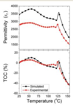
Fig. 6 Overlaid FEM simulation models and experimental data of temperature profiles for (a)  $\varepsilon_r$  and (b) TCC. Excellent agreement is obtained showing the prediction of combining a BT core with 2.5% doped NNBT with  $V_f = 0.66$  provides potentially useful TCC behaviour.
