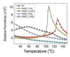
Fig. 1 Permittivity (100 kHz) versus temperature profiles for  $x(NaNbO_3)-(1 - x)BaTiO_3$  (NNBT, x = 0, 0.01, 0.025, 0.05, 0.10) ceramics
