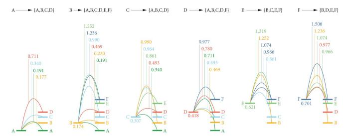
Fig. 6 Calculated energy barriers for vacancy diffusion between each site. Schematic of the calculated minimum energy barriers for all Li-Li site vacancy hops with site separations ≤4 Å. All energies are in eV, and give the maximum energy along each minimum-energy path relative to the energy of a vacancy at site Li<sup>A</sup>. Relative energies of vacancies at sites Li<sup>(B-F)</sup> are also given.
