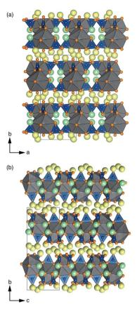
Fig. 1 Crystal structure of  $\text{Li}_6 Y (\text{BO}_3)_3$ . Illustration of the crystal structure of monoclinic  $\text{Li}_6 Y (\text{BO}_3)_3$  viewed along the (a) c- and (b) a-axis. B is shown in blue, Y in gray, O in orange, and Li in yellow or green. Edgesharing  $\text{YO}_8$  dodecahedra form chains that zig-zag along the c-axis. Trigonal bipyramidal chains of  $\text{LiO}_5$  form along the c-direction and connect the chains of  $\text{YO}_8$  along the a-direction.
