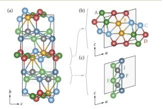
Fig. 5 Illustration of the Li sites with respect to each other. Illustration of the various Li positions with respect to each other viewed down the (a) c-axis, (b) with the Li-rich layer, and (c) within the 1D chains.
