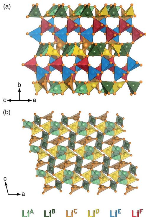
Fig. 2 Local coordination environment of each Li site in  $\text{Li}_6\text{Y}(\text{BO}_3)_3$ . Illustration of the polyhedral connectivity between the six neighboring Li positions viewed along the (a) [101] and (b) [010] unit cell directions. There are two distinct topologies in the structure: the edge sharing ribbons of  $\text{Li}^{\text{E}}$  and  $\text{Li}^{\text{F}}$  and the layers of  $\text{Li}^{\text{A-D}}$ . For clarity, Y and B are not shown.
