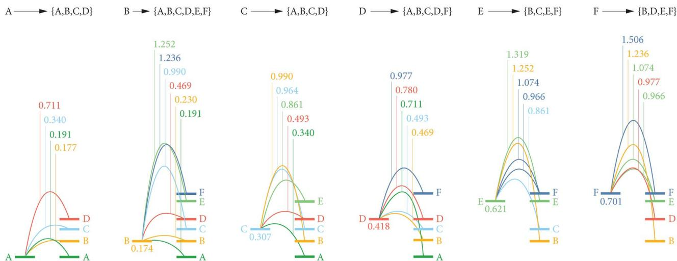
Fig. 6 Calculated energy barriers for vacancy diffusion between each site. Schematic of the calculated minimum energy barriers for all Li–Li site vacancy hops with site separations  $\leq 4$  Å. All energies are in eV, and give the maximum energy along each minimum-energy path relative to the energy of a vacancy at site  $\text{Li}^A$ . Relative energies of vacancies at sites  $\text{Li}^{(B-F)}$  are also given.
