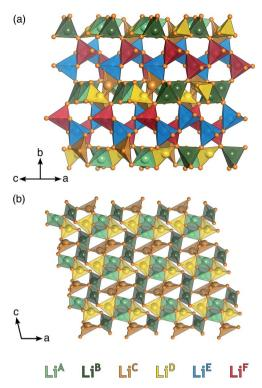
Fig. 2 Local coordination environment of each Li site in Li<sub>6</sub>Y(BO<sub>3</sub>)<sub>3</sub>. Illustration of the polyhedral connectivity between the six neighboring Li positions viewed along the (a) [101] and (b) [010] unit cell directions. There are two distinct topologies in the structure: the edge sharing ribbons of Li<sup>E</sup> and Li<sup>F</sup> and the layers of Li<sup>A-D</sup>. For clarity, Y and B are not shown
