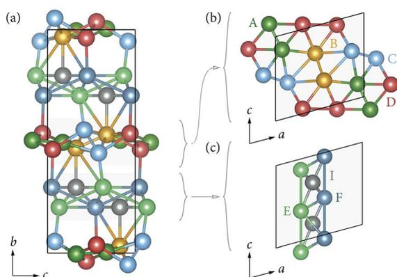
Fig. 5 Illustration of the Li sites with respect to each other. Illustration of the various Li positions with respect to each other viewed down the (a) *c*-axis, (b) with the Li-rich layer, and (c) within the 1D chains.
