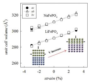
Fig. 2 Change in the calculated unit cell volume as a function of strain for LiFePO $_4$  and NaFePO $_4$  together with a schematic representation of the effect of compressive (<0%) or tensile (>0%) lattice strain on the thin film system.
