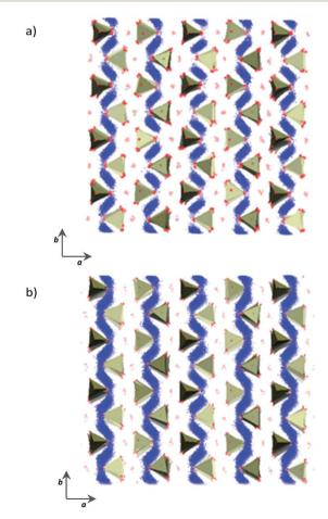
Fig. 5 Na-ion trajectory plot for (a) unstrained Na<sub>0.9</sub>FePO<sub>4</sub> and (b) 3% ac-strained Na<sub>0.9</sub>FePO<sub>4</sub> showing the Na-ion zig-zag path. Projection along the c axis. Blue spheres represent the positions occupied by Na ions over the simulation time; pink spheres represent the Fe ions in their final configuration while the tetrahedra represent the PO<sub>4</sub> units.
