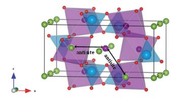
Fig. 7 Schematic representation of two configurations of Li/Fe or Na/Fe anti-site defects in olivine-type AFePO<sub>4</sub> ( $A = Li^+$  or Na<sup>+</sup>).
