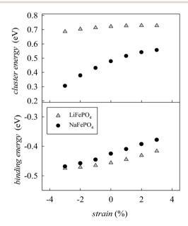
Fig. 8 Anti-site defect energies for olivine-type AFePO<sub>4</sub> ( $A = Li^+$  or Na $^+$ ) as a function of the applied biaxial tensile/compressive strain in the ac plane; (upper) cluster formation energy (based on eqn (1) and (2)); (lower) binding energy.
