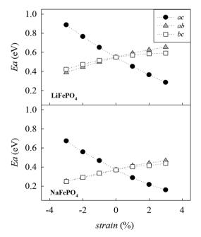
Fig. 4 Change in the alkali-ion migration barrier along the [010] direction as a function of strain for LiFePO<sub>4</sub> (upper panel) and NaFePO<sub>4</sub> (lower panel).
