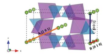
Fig. 3 Schematic representation of the possible migration paths in olivine-type AFePO<sub>4</sub> ( $A = Li^+$  or  $Na^+$ ). Blue: PO<sub>4</sub> tetrahedra; purple: FeO<sub>6</sub> octahedra; green: Li/Na.
