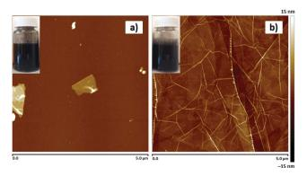
Fig. 1 AFM images ( $5 \times 5 \, \mu m^2$ ) of chemically reduced graphene oxide (CRGO) (a) without and (b) with SDBS. Insets show digital photographs of the corresponding samples in an aqueous 1 mg mL<sup>-1</sup> solution.
