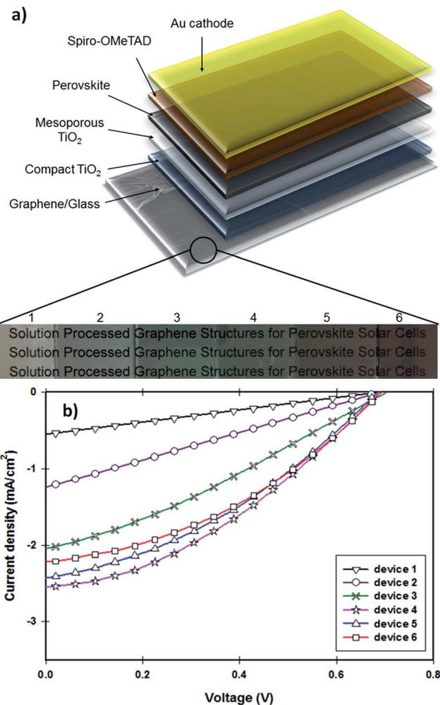
Fig. 5 (a) Device structure, (b) photocurrent density–voltage ( $J$ – $V$ ) curve of the fabricated solar cells with transparent graphene electrodes. PSC devices with  $0.075 \text{ cm}^2$  active area were illuminated under AM 1.5G simulated sunlight ( $100 \text{ mW cm}^{-2}$ ).
