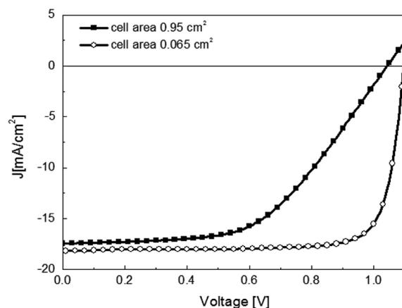
Fig. 6  $J$ - $V$  curves for the optimized  $\text{CH}_3\text{NH}_3\text{PbI}_3$  perovskite layer with a small ( $A = 0.065 \text{ cm}^2$ ) and larger ( $A = 0.95 \text{ cm}^2$ ) electrode size. The solar cell in planar heterojunction architecture is composed by ITO/PEDOT:PSS/PolyTPD/ $\text{CH}_3\text{NH}_3\text{PbI}_3$ /PCBM/3TPYMB/Au. Reproduced with permission from ref. 71.
