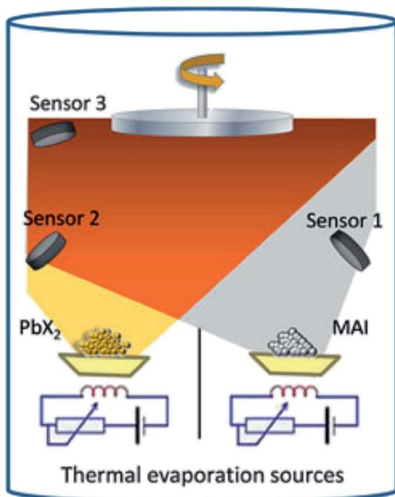
Fig. 4 Illustration of the dual-source vacuum deposition instrument. The  $\text{PbX}_2$  ( $X = \text{I}, \text{Cl}$ ) and  $\text{CH}_3\text{NH}_3\text{I}$  (MAI) precursors are thermally evaporated in vacuum. The deposition rate and thickness are monitored using quartz microbalances. Reproduced with permission from ref. 75.
