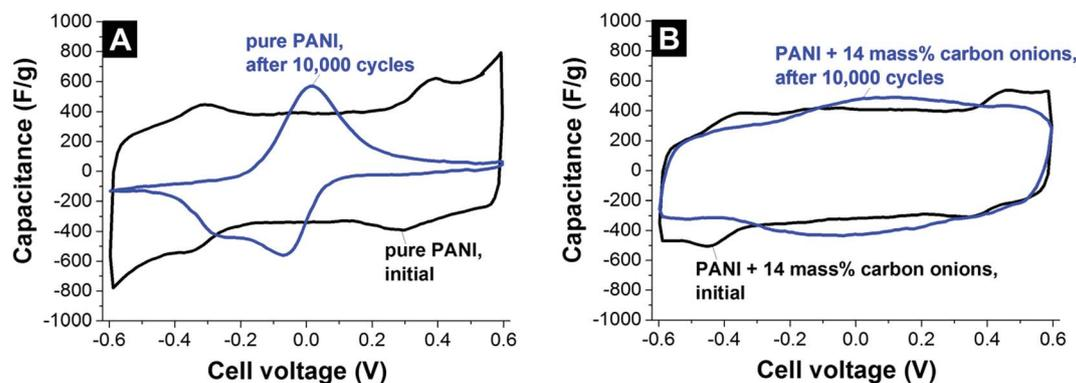
Fig. 15 Cyclic voltammograms of nanodiamond-derived carbon onions ( $1800 \text{ }^\circ\text{C}$  synthesis temperature) coated with PANI. Electrodes are PTFE-bound (3 mass%) and measured in a two-electrode configuration using  $1 \text{ M H}_2\text{SO}_4$  recorded at a scan rate of  $1 \text{ mV s}^{-1}$ . (A) Pure PANI electrodes. (B) Carbon onion/PANI composite with 14 mass% carbon onions. Data adapted from ref. 132.
