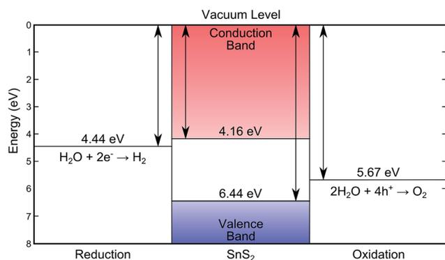
Fig. 4 The energy levels of SnS<sub>2</sub> as determined by XPS/IPES in this work, showing the desirable band placements for water splitting.<sup>7,8</sup>
