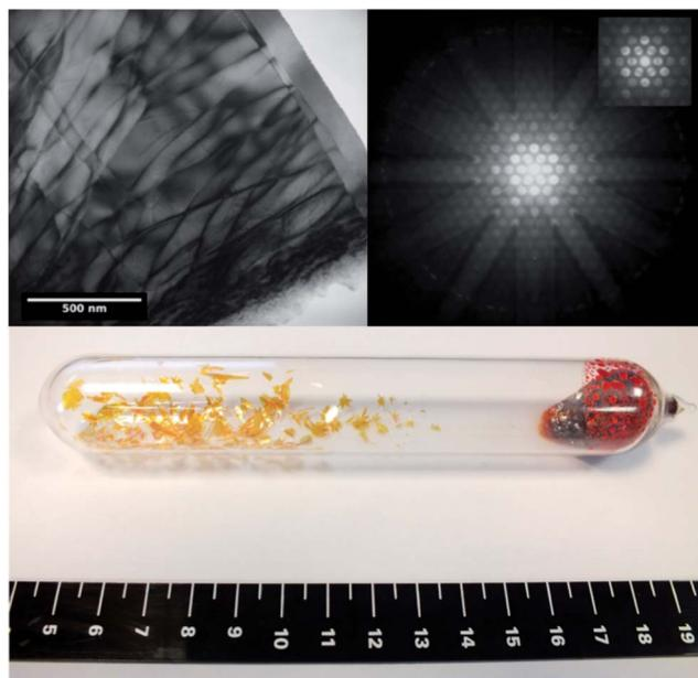
Fig. 2 Top left – Bright field transmission electron microscopy of an SnS<sub>2</sub> platelet, image near the [0001] zone axis. Top right – Convergent beam electron diffraction pattern near the [0001] zone axis and, inset, detail of the zero order Laue zone from the same sample. Bottom centre – Macroscopic single crystals synthesised from the CVT method, with the scale in centimetres.
