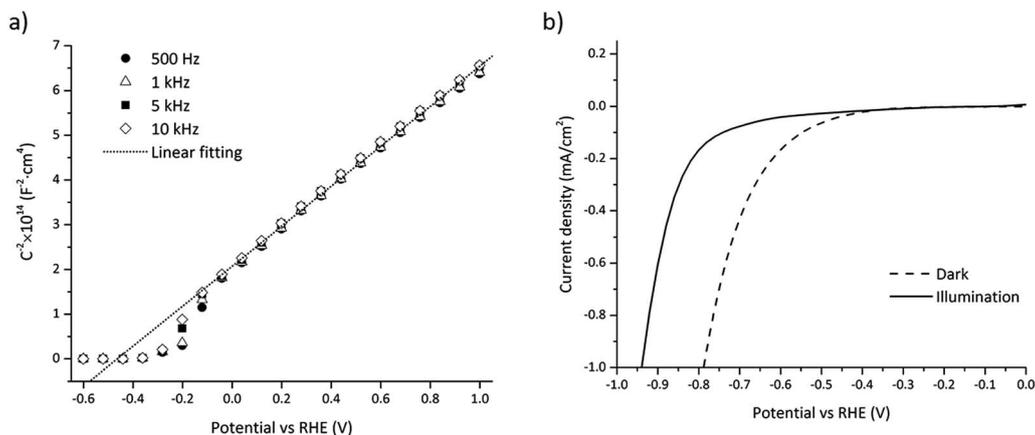
Fig. 5 (a) Mott–Schottky plot for four frequencies (500 Hz, 1 kHz, 5 kHz, 10 kHz) of a 1  $\mu\text{m}$  thick *ni*-GaN sample immersed in 1 M  $\text{H}_2\text{SO}_4$  electrolyte under dark. (b) Experimental dark current density (dashed line) and photocurrent density (solid line) vs. RHE.
