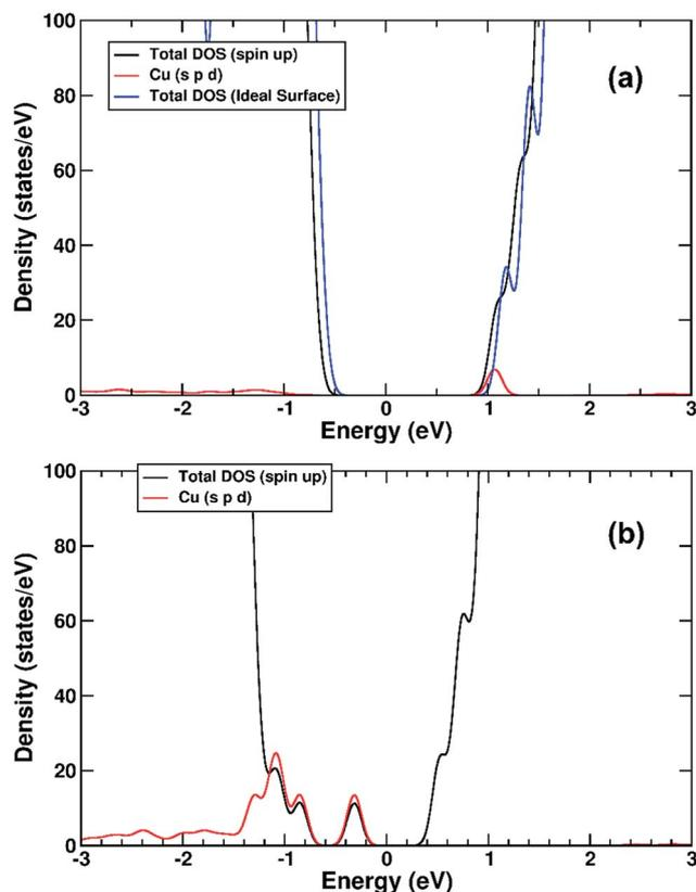
Fig. 10 (a) DOS of the  $\text{TiO}_2(\text{R})\text{-Cu}$  system, spin-up channel only, aligned to the DOS of the ideal  $\text{TiO}_2(\text{R})$  surface. (b) The spin up channel DOS of the final relaxed electron polaron system for the  $\text{TiO}_2(\text{R})\text{-Cu}$  system. Cu contribution shown. The zero of the x-axis is fitted to the VBM for both plots.
