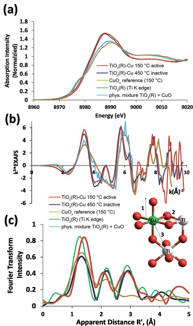
Fig. 4 XAS spectra of photocatalytically active  $\text{TiO}_2(\text{R})$ -Cu (dried at 150 °C) and inactive  $\text{TiO}_2(\text{R})$ -Cu (calcined at 450 °C) are compared to the reference data of  $\text{CuO}_x$  (prepared by heating), rutile  $\text{TiO}_2(\text{R})$  (Ti K edge), and a physical mixture of  $\text{TiO}_2(\text{R})$  and CuO. Data are presented as XANES (a), EXAFS (b) and Fourier transform of the EXAFS (c). The inset shows a structural model used for fitting.
