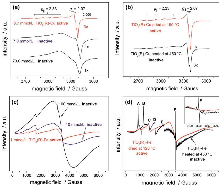
Fig. 5 EPR spectra of photocatalytically active and inactive  $\text{TiO}_2(\text{R})\text{-Cu}$  (a) and  $\text{TiO}_2(\text{R})\text{-Fe}$  (c) powders prepared using different concentrations of metal ion precursors; change of EPR spectra of  $\text{TiO}_2(\text{R})\text{-Cu}$  (b) and  $\text{TiO}_2(\text{R})\text{-Fe}$  (d) upon heat treatment at  $450\text{ }^\circ\text{C}$ .
