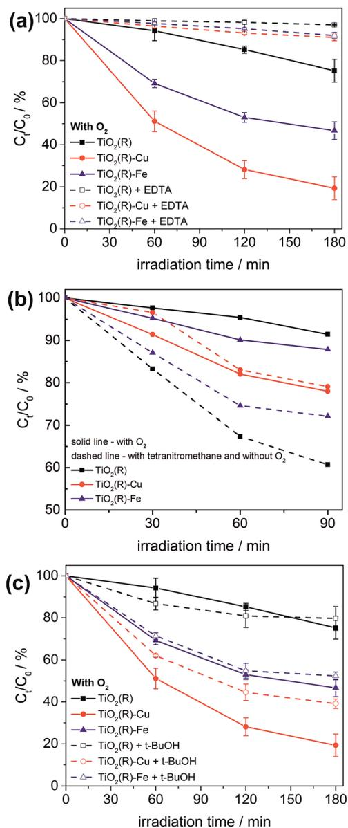
Fig. 11 Comparison of 4-CP degradation yields during photocatalytic degradation experiments using suspensions of  $TiO_2(R)$ ,  $TiO_2(R)-Cu$  and  $TiO_2(R)-Fe$  under different conditions: in the presence or absence of oxygen and in the presence of scavengers: (a) EDTA (holes), (b) tetranitromethane (electrons), (c) and *tert*-butanol (OH radicals). Note that the experiments in (b) have been performed in a reactor setup different from (a) and (c).
