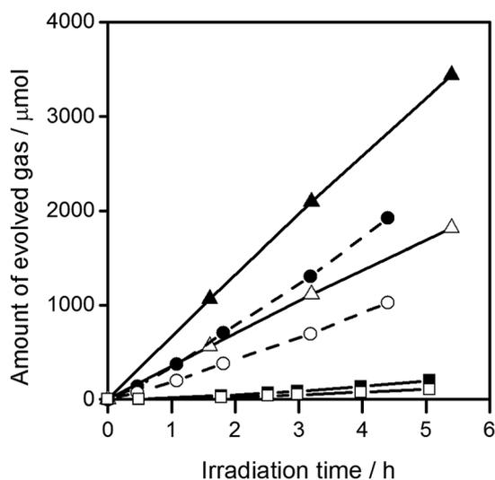
Fig. 5 Gas evolution during the water splitting reaction on Al-STO(-flux-Y). H<sub>2</sub> (■) and O<sub>2</sub> (□) on 0.1%Al-STO(flux-Y), H<sub>2</sub> (●) and O<sub>2</sub> (○) on 1%Al-STO(flux-Y), and H<sub>2</sub> (▲) and O<sub>2</sub> (△) on 10%Al-STO(flux-Y). Reaction conditions: catalyst, 0.1 g; cocatalyst, Rh<sub>2-y</sub>Cr<sub>y</sub>O<sub>3</sub> (Rh 0.1 wt%, Cr 0.1 wt%); reaction solution, 100 mL H<sub>2</sub>O; light source, 300 W Xe lamp (λ > 300 nm).
