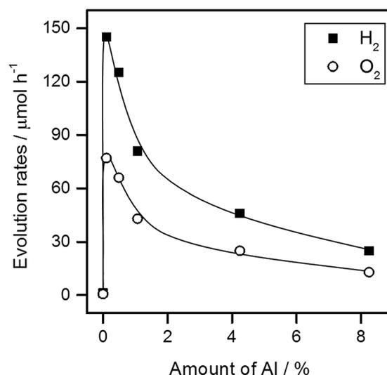
Fig. 6 Dependence of the water splitting activity of STO(ssr-Y) on the amount of Al doping. Reaction conditions: catalyst, 0.1 g; cocatalyst, Rh<sub>2-y</sub>Cr<sub>y</sub>O<sub>3</sub> (Rh 0.1 wt%, Cr 0.1 wt%); reaction solution, 100 mL H<sub>2</sub>O; light source, 300 W Xe lamp (λ > 300 nm).
