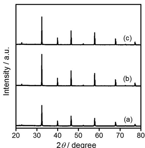
Fig. 1 XRD patterns for SrTiO<sub>3</sub> particles. (a) STO(pristine), (b) STO(flux-Y), and (c) STO(flux-Al).
