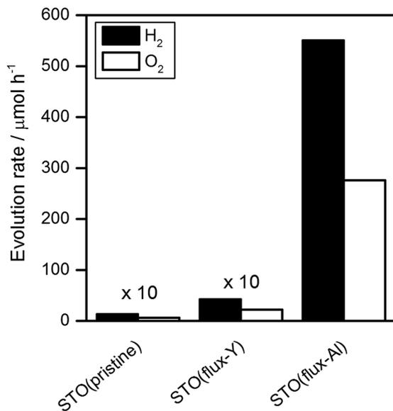
Fig. 3 Water splitting activity of SrTiO<sub>3</sub> photocatalysts. Reaction conditions: catalyst, 0.1 g; cocatalyst, Rh<sub>2-y</sub>Cr<sub>y</sub>O<sub>3</sub> (Rh 0.1 wt%, Cr 0.1 wt%); reaction solution, 100 mL H<sub>2</sub>O; light source, 300 W Xe lamp ( $\lambda > 300$  nm).
