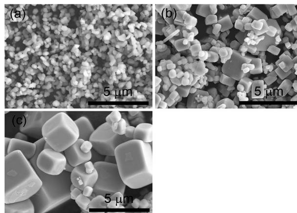
Fig. 2 SEM images of SrTiO<sub>3</sub> particles. (a) STO(pristine), (b) STO(flux-Y), and (c) STO(flux-Al).
