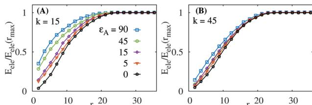
Fig. 5 Total elastic energy of the lattice deformations versus the physical distance  $r$  from the centre of a single rod for a range of adhesion strength  $\epsilon_A$ . The results are normalised to the overall network energy. Elastic constants and attraction energies are indicated.
