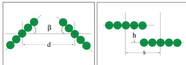
Fig. 1 Rotation and sliding scheme of membrane-adhered rods (view from the top). Here, for rotating rods  $\beta$  designates the mutual orientation angle and  $d$  is the particle–particle distance with respect to their centre of mass. For sliding rods,  $h$  is the inter-axial separation between the particles (offset distance) and  $s$  is the sliding distance.
