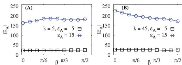
Fig. 6 Total rod-network adsorption energy  $E_A$  versus the rod-rod mutual orientation angle  $\beta$ , plotted for different sheet stiffness  $k$  and rod-network attraction  $\epsilon_A$ . The left panel represents softer sheets. Larger rod-substrate attractions on stiffer sheets yield a stronger  $E_A(\beta)$ -dependence (right panel). Parameters are the same as in Fig. 5.
