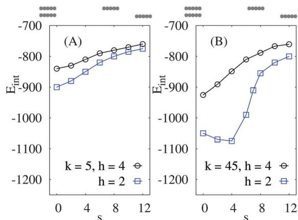
Fig. 10 Interaction energy of two rods sliding along each other at fixed inter-axial offset  $h$  and varying distance  $s$ , as indicated on the top of each panel. Parameters:  $\epsilon_A = 15$ ,  $n = 25$ . The energy values for large  $s$  and small  $h$  approach those for  $d = s$  inter-rod separations shown in Fig. 8.
