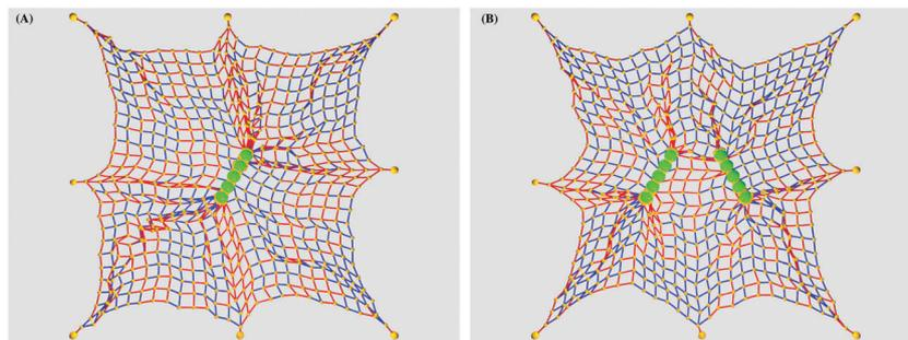
Fig. 3 Network deformation pattern in the vicinity of a single rod and two rods with simultaneously varied mutual angle  $\beta_1 = \beta_2 = \beta$ , evaluated at a single time moment for the parameters of Fig. 2.
