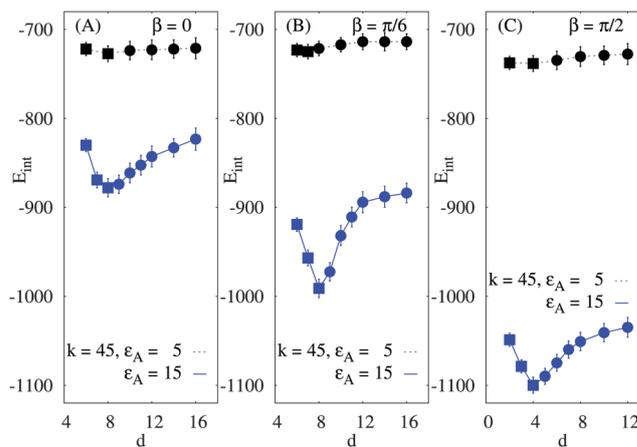
Fig. 8 Interaction energy  $E_{\text{int}}(d)$  of substrate-adsorbed rods versus inter-axial distance  $d$ , plotted for  $\beta = 0, \pi/6$ , and  $\pi/2$  (from left to right). Other parameters are indicated in the plots. The circles and squares designate the regions of attraction and repulsion, respectively. The error bars are shown.
