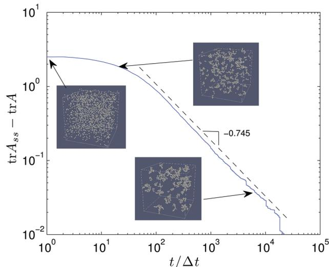
Fig. 2 Log-log plot of  $\text{tr}\mathbf{A}_{ss} - \text{tr}\mathbf{A}$  vs. time shows power-law evolution of  $\text{tr}\mathbf{A}$  to steady state in the absence of external shearing. Inset images (for illustration purposes only) from a highly dilute simulation demonstrate the aggregation of particles into clusters in the simplified discrete model. Clusters in the simulation used to generate the curve span the domain after a short period of aggregation, forming conductive networks.
