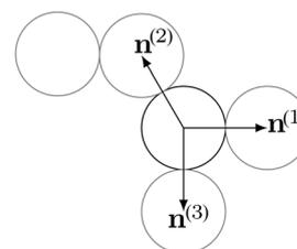
Fig. 1 Schematic of particles in contact showing unit contact normal vectors  $\mathbf{n}_i$  for computation of the fabric tensor.
