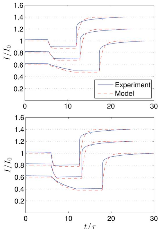
Fig. 7 Transient ramp experiments reproduced with the evolution law with  $n = 0$ . The model fails to adequately capture the relaxation behavior that occurs upon cessation of flow.
