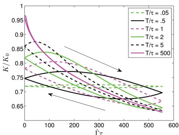
Fig. 9 Plot of normalized stable conductivity loops that are formed during cyclic shear rate simulations for six different cycle periods. Arrows indicate the progression of time along each side of the cycle.
