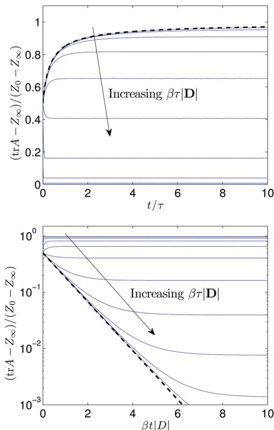
Fig. 6 Evolution of  $Z = \text{tr}\mathbf{A}$  in pure shearing under different shear rates, as predicted by the model. (top)  $\beta\tau|\mathbf{D}| \ll 1$  yields power-law approach of  $Z$  to steady state;  $|Z - Z_0| \sim t^{-1/n}$  as  $|\mathbf{D}| \rightarrow 0$ , dotted line. (bottom)  $\beta\tau|\mathbf{D}| \gg 1$  yields exponential approach to steady state;  $\log(Z - Z_\infty) \sim -|\mathbf{D}|t$  as  $|\mathbf{D}| \rightarrow \infty$ , dotted line.
