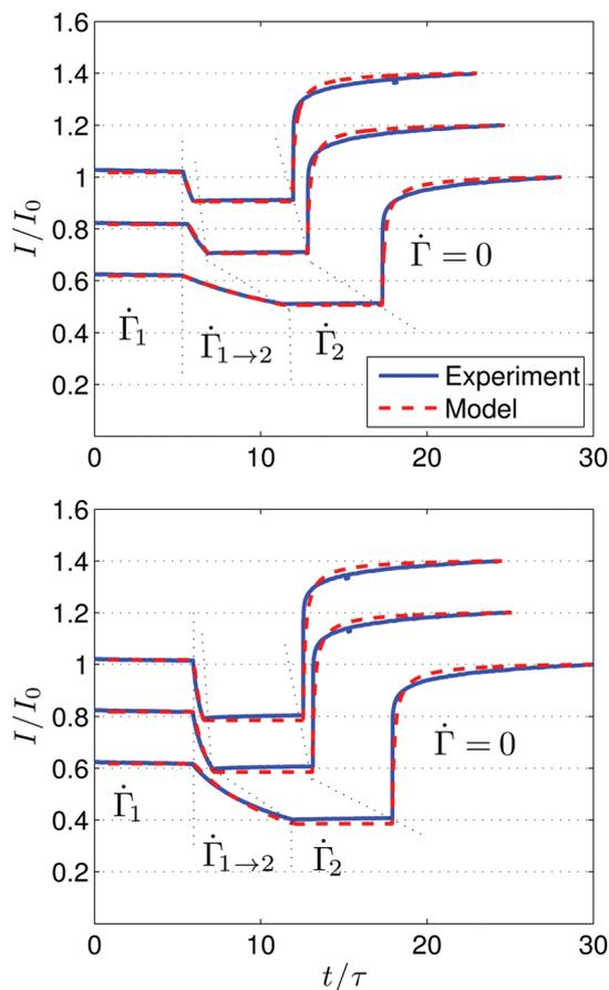
Fig. 5 Transient ramp experiments from (top)  $\tau \dot{\Gamma}_1 = 2500$  to  $\tau \dot{\Gamma}_2 = 5000$ , and (bottom)  $\tau \dot{\Gamma}_1 = 2500$  to  $\tau \dot{\Gamma}_2 = 10000$  with ramp times  $t_R/\tau$  of 0.6, 1.2, and 6 (top to bottom). A vertical offset of 0.2 has been added between successive curves for clarity, with the y-axis correct as displayed for the bottom curve. Current values are normalized by the static current measurement  $I_0$ .
