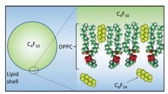
Fig. 8 Schematic diagram showing (i) the incorporation of  $C_6F_{14}$  into the MB shell thereby reducing surface tension and the Laplace driving force for dissolution and (ii) the saturation of the medium with  $C_6F_{14}$  thereby reducing the solubility of  $C_4F_{10}$  in the ambient phase.
