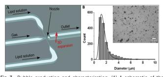
Fig. 3 Bubble production and characterisation. (A) A schematic of the microfluidic chip design emphasizing the 3D expansion region for the production of MBs in the spray regime. (B) Graph displaying the size distribution for one of the bubble populations. The inset shows a bright field image representing the produced MBs (sample is 10-fold diluted).
