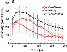
Fig. 5 Ultrasound time intensity curves in mice aorta. (A) shows the effect of increasing the final lipid concentration, and saturating the lipid solution with  $C_6F_{14}$  on MB lifetime for MBs made with DPPC + 5% PEG $_{2000}$  and encapsulating  $C_4F_{10}$  gas. (B) compares TIC curves for our improved in-house MBs and commercial MBs.
