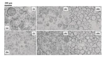
Fig. 7 (upper) Photographs after 1 month of (a) sunflower oil-in-50 cS PDMS-in-sunflower oil and (b) olive oil-in-50 cS PDMS-in-olive oil multiple emulsions containing a volume fraction of initial V/S emulsion of (i) 0.3 and (ii) 0.7 prepared using low shear; (iii) simple V/S emulsions containing the vegetable oils and 50 cS PDMS after attempting to prepare S/V/S multiple emulsions with low shear. (lower) Corresponding optical micrographs of the emulsions.
