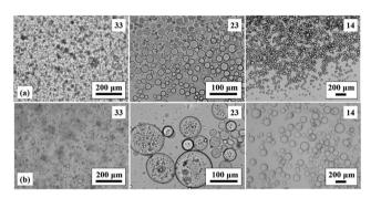
Fig. 3 Corresponding optical micrographs of the emulsions shown in Fig. 2 at selected % SiOH (given) for (a) sunflower oil and (b) olive oil with DCDMS-coated particles
