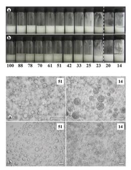
Fig. 5 (upper) Photographs of glass vials containing (a) sunflower oil-100 cS PDMS and (b) olive oil–100 cS PDMS emulsions (both 1:1) after 1 month stabilised by 1 wt% of DCDMS-coated fumed silica particles with different % SiOH on their surfaces (given). Dashed line indicates transitional phase inversion. (lower) Corresponding optical micrographs of the emulsions at selected % SiOH (given). Scale bars = 200 μm.
