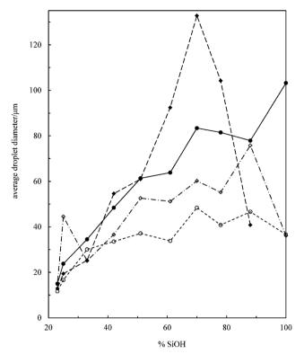
Fig. 6 Plot of average droplet diameter of 50 cS PDMS-in-sunflower oil ( $\bullet$ ), 100 cS PDMS-in-sunflower oil ( $\circ$ ), 50 cS PDMS-in-olive oil ( $\bullet$ ) and 100 cS PDMS-in-olive oil ( $\circ$ ) emulsions after 1 month *versus* % SiOH on DCDMS-coated fumed silica particle surfaces. Standard deviation is in the range of 30  $\mu$ m at relatively high % SiOH and 10  $\mu$ m at relatively low % SiOH.
