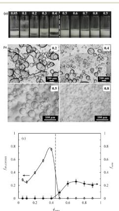
Fig. 11 (a) Photograph after 1 month of glass vials containing sunflower oil-50 cS PDMS emulsions stabilised by 1 wt% of 75% SiOH fluorinated silica particles containing varying volume fraction of sunflower oil  $\phi_{ extsf{suno}}$ (given). Emulsions are V/S (left) and S/V (right) either side of the dashed line. (b) Corresponding optical micrographs of the emulsions at selected  $\phi_{
