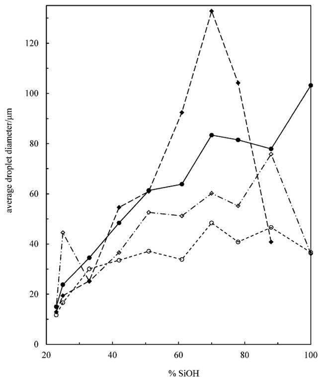
Fig. 6 Plot of average droplet diameter of 50 cS PDMS-in-sunflower oil (●), 100 cS PDMS-in-sunflower oil (○), 50 cS PDMS-in-olive oil (◆) and 100 cS PDMS-in-olive oil (◇) emulsions after 1 month versus % SiOH on DCDMS-coated fumed silica particle surfaces. Standard deviation is in the range of 30  $\mu\text{m}$  at relatively high % SiOH and 10  $\mu\text{m}$  at relatively low % SiOH.
