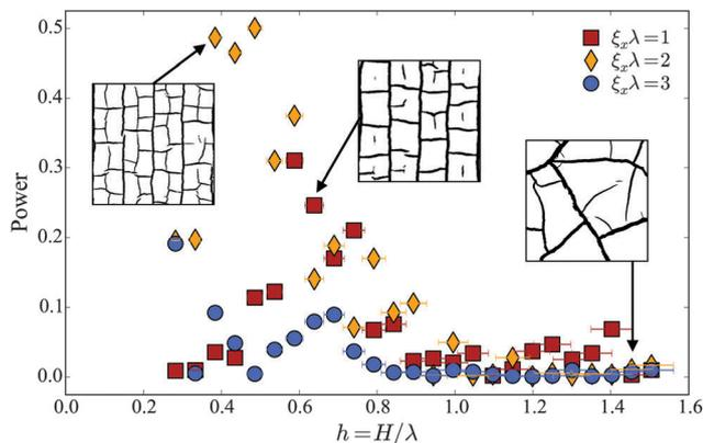
Fig. 7 Spectral power of the lowest-order peaks for cracks over plate 2. At  $h = 0.6$  there is a transition from a pattern with cracks along the peaks and troughs of the substrate, to one with cracks only along the peaks. Insets show  $4 \times 4 \text{ cm}^2$  samples of crack patterns from the indicated conditions.
