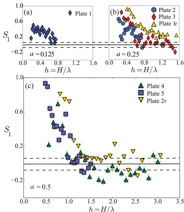
Fig. 9 The orientational order parameter  $S_1$  (eqn (1)) describes how well-aligned individual peds (continuous regions, entirely bounded by cracks) are with the orientation of their substrate. Results are given for wave plates with dimensionless amplitudes (a)  $a = 0.125$ , (b)  $a = 0.25$  and (c)  $a = 0.5$ . The solid and dashed lines represent the mean and standard deviation of measurements of  $S_1$  on flat plates.
