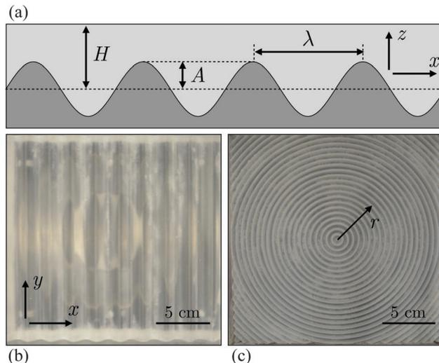
Fig. 2 Sketch of the drying experiment, where (a) a clay slurry of average initial thickness  $H$  dries over a sinusoidally varying substrate, of amplitude  $A$  and wavelength  $\lambda$ . Both (b) linear and (c) radial wave plates were used as substrates.
