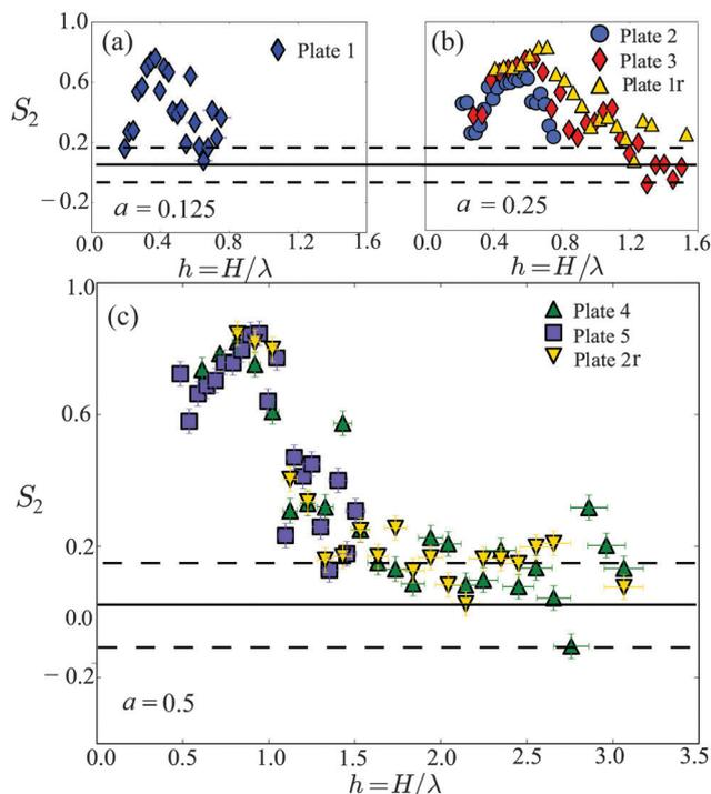
**Fig. 11** The crack alignment order parameter  $S_2$  (eqn (2)) measures the relative alignment of cracks with their substrate, and takes large values for networks with cracks that are parallel or perpendicular to the underlying relief. Shown are the results for (a)  $a = 0.125$ , (b)  $a = 0.25$ , and (c)  $a = 0.5$ . The solid and dashed lines represent the mean and standard deviation of  $S_2$  for cracks over the flat plate.
