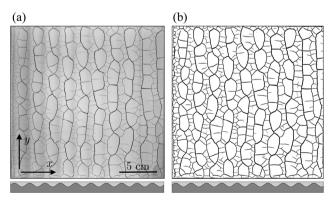
Fig. 3 Image processing. Each image (a) is cropped, contrast-adjusted, filtered and thresholded to (b) yield a black-and-white description of the crack positions. The shape of the substrate (plate 1) is sketched below
