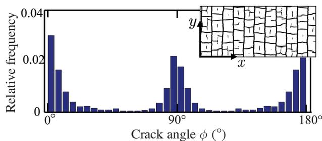
Fig. 10 The distribution of crack orientations in a ladder-like pattern. The peak at  $0^\circ$  and  $180^\circ$  (these two angles being equivalent) reflects the dominant cracks parallel to the  $y$ -axis, while the peak at  $90^\circ$  comes from the shorter 'rungs' of the ladders.
