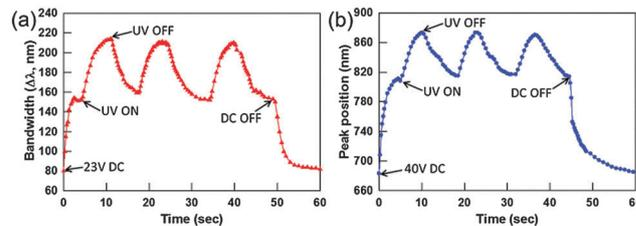
Fig. 4 Photoinduced changes (on/off) with exposure to (a)  $60 \text{ mW cm}^{-2}$  of bandwidth broadening in b-PSCLC at 23 V DC and (b)  $40 \text{ mW cm}^{-2}$  of tuning of t-PSCLC at 40 V DC.
