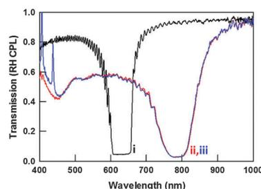
**Fig. 8** Photosensitivity of t-PSCLC prepared with the photoinitiator I-651 (1 wt%). Transmission spectra at (i) 0 V (—), (ii) during application of 45 V DC (—), and (iii) during application of 45 V DC in the presence of 70 mW cm<sup>-2</sup> of UV light (—).
