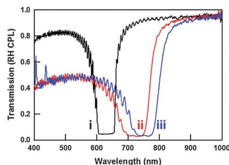
**Fig. 7** Photosensitivity of t-PSCLC prepared with the photoinitiator I-907 (1 wt%). Transmission spectra at (i) 0 V (—), (ii) during application of 40 V DC (—), and during application of 40 V DC in the presence of 50 mW cm<sup>-2</sup> of UV light (—).
