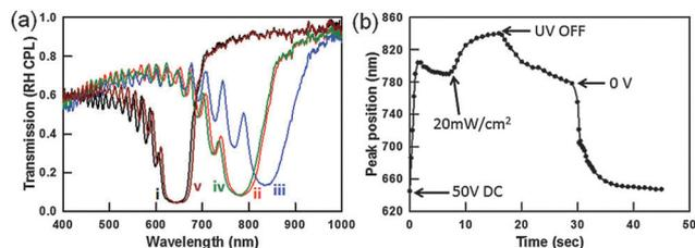
Fig. 3 (a) Transmission (RH circularly polarized probe light) spectra of t-PSCLC (i) before (—), (ii) during application of 50 V DC (—), (iii) during application of 50 V DC and  $20 \text{ mW cm}^{-2}$  of UV light (—), (iv) after removal of UV light (50 V DC maintained) (—), and (v) after removal of 50 V DC (—). (b) Temporal response of t-PSCLC to initial application of 50 V DC, exposure to  $20 \text{ mW cm}^{-2}$ , after removal of UV light, and after removal of 50 V DC.
