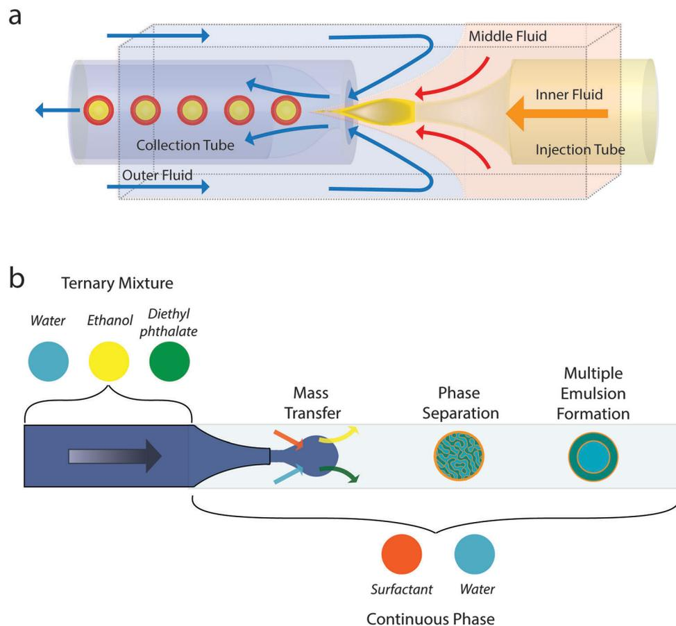
**Fig. 3** (a) Schematic showing the microfluidic production of multiple emulsions using combined co-flow and flow focusing in a single device. Adapted from ref. 27. (b) Schematic showing the microfluidic production of multiple emulsions using combining droplet production using flow focusing with phase separation. Based on description in ref. 35.
