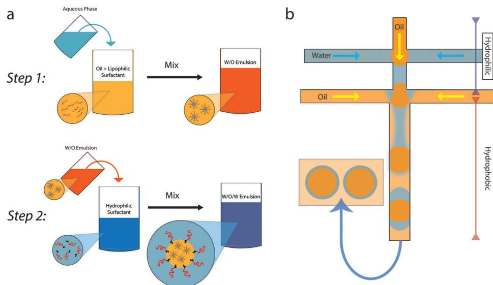
**Fig. 1** Schematics showing the two step production of a multiple emulsion. (a) Conventional batch emulsification: step 1 is creating the internal droplets, step 2 creates the outer droplets using gentle shear. Adapted from ref. 1 with permission from Elsevier. (b) Step-wise production of multiple emulsions using microfluidics. Successive junctions are used to create the internal and external droplets. (This apparatus can be adapted for one-step emulsification.<sup>82</sup>)
