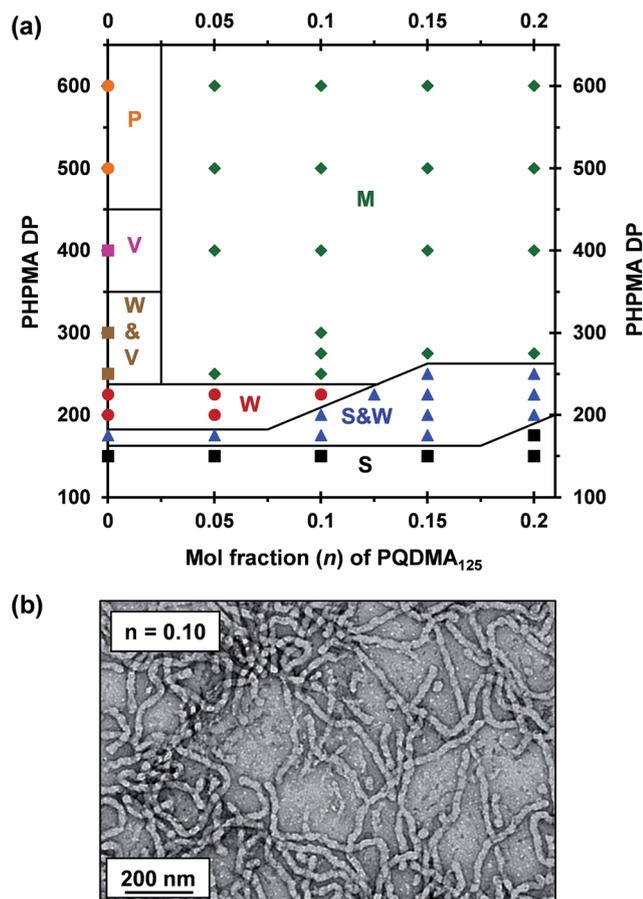
Fig. 1 (a) Phase diagram constructed for the RAFT aqueous dispersion polymerization of HPMA at a fixed copolymer concentration of 20% w/w solids at 50 °C using a binary mixture of PEO<sub>113</sub>-PETTC and PQDMA<sub>125</sub> macro-CTAs [S = spheres, W = worms, V = vesicles, M = mixed phase and P = precipitate]. (b) Representative TEM image for linear cationic (0.9PEO<sub>113</sub> + 0.1PQDMA<sub>125</sub>)-PHPMA<sub>225</sub> worms.
