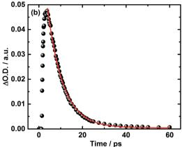
Fig. 5 (a) Transient absorption spectra of 5 in argon-saturated THF upon fs-laser photolysis (568 nm, 400 nJ per pulse) with time delays 2 ps (black), 5 ps (red), 10 ps (green), 25 ps (blue), and 100 ps (cyan) after the laser pulse. (b) Corresponding time absorption profile (black) and exponential decay fit (red) at 590 nm.
