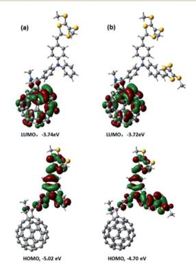
Fig. 3 Optimized structures and electron densities of LUMOs and HOMOs of (a) 4 and (b) 5 calculated at the B3LYP/3-21G level of theory.
