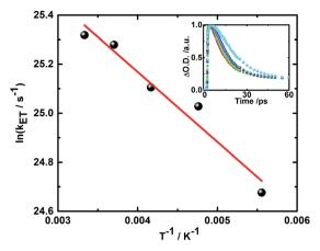
Fig. 6 Plot of rate constant for the charge recombination of the singlet radical ion pair state  $vs. T^{-1}$  for 5 in 2-methyl THF upon photoexcitation at 387 nm. Linear fit is shown in red. Inset: corresponding time-absorption profiles at 600 nm obtained at 300 K (black), 270 K (red), 240 K (green), 210 K (blue), and 180 K (cyan).
