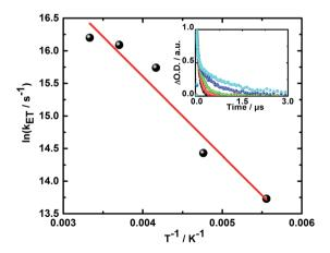
Fig. 7 Plot of the rate constant for the charge recombination of the triplet radical ion pair state  $vs.\ T^{-1}$  for 5 in 2-methyl THF upon photoexcitation at 387 nm. Linear fit is shown in red. Inset: corresponding time-absorption profiles at 600 nm obtained at 300 K (black), 270 K (red), 240 K (green), 210 K (blue), and 180 K (cyan).
