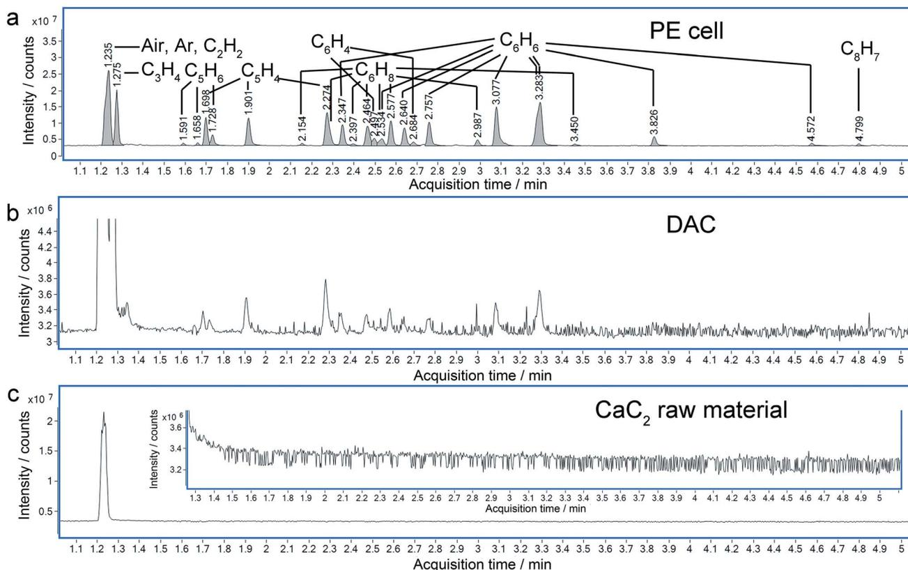
Fig. 7 Total ion chromatograms (TIC) of the product of  $\text{CaC}_2$  recovered from 26 GPa and  $\text{CaC}_2$  raw material reacting with water. (a) Sample synthesized by PE cell. (b) Sample synthesized by DAC. (c)  $\text{CaC}_2$  raw material (before compression).
