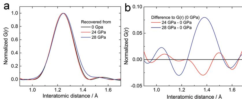
Fig. 6 Neutron pair distribution functions ( $G(r)$ ) of  $\text{CaC}_2$  samples recovered from external pressures. (a) Selected normalized first peak after background subtraction. This peak corresponds to the carbon–carbon bond. (b) Differences between the normalized  $G(r)$  patterns of the samples recovered from high pressure (24 GPa, 28 GPa) and that of the raw material (0 GPa).
