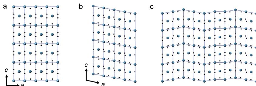
Fig. 3 Structures of  $\text{CaC}_2$ -I (a) and VI (b) viewed along [010]; (c) a schematic model of possible local disordering of  $\text{CaC}_2$  above 12 GPa. The black spheres are for carbon atoms and the blue spheres are for calcium atoms.
