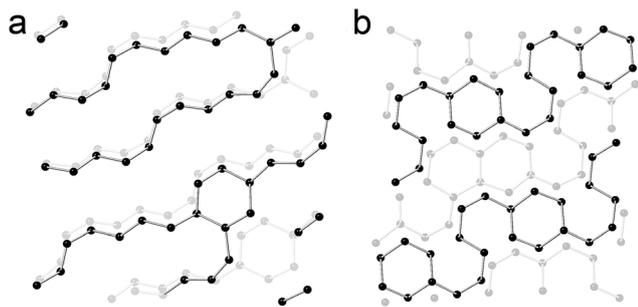
Fig. 8 Simulated structure of  $\text{CaC}_2$  at 30 GPa by meta-dynamics. (a) Chain model. (b) Ribbon model. The C–C bond limitation is set at 1.6 Å. Ca ions are omitted for clarity.
