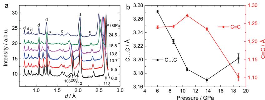
Fig. 2 *In situ* neutron diffraction patterns of  $\text{CaC}_2$  under different values of pressure. (a) Neutron diffraction patterns of  $\text{CaC}_2$  under high pressure. The peaks of diamond anvils and  $\text{CaO}$  are marked by d and c respectively. (b) C–C bond length and the nearest C...C distance between neighbouring  $\text{C}_2^{2-}$  units under different values of external pressure.
