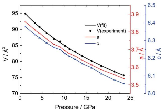
Fig. 1 Lattice parameters of CaC<sub>2</sub> under high pressure. The red and blue markers including error bars are for the *a* and *c*-axis respectively, and the lines are a guide for the eyes. The black dots are the experimental data of the unit cell volume, and the black solid line is the fitting of the BM-EOS.
