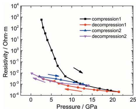
Fig. 9 Pressure dependent electrical resistivity of  $\text{CaC}_2$ .
