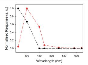
Fig. 8 Comparison of normalised photocurrent of xerogel-1,2 (red), and xerogel-1 (black data) at different wavelengths. The responses were measured at 4 V using a 2 electrode set up, see Fig. S8 and S9.† Data at the different wavelengths were collected for the same samples at different wavelengths after allowing full recovery to baseline before a new measurement was carried out.
