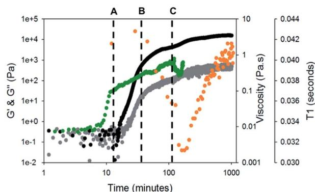
Fig. 4 Comparison of change in  $G'$  and  $G''$  over time for gel-1,2 (black data are  $G'$  and grey data are  $G''$ ) to change in viscosity (green data) whilst gelling. Orange data are the  $T_1$  relaxation time of  $^{23}\text{Na}^+$  over time. Time sweeps were performed at a strain of 0.5%, 10  $\text{rad s}^{-1}$  and at 25  $^\circ\text{C}$ . Viscosity measurements were performed at 5  $\text{s}^{-1}$ . For discussion around points A, B, and C, please see main text.
