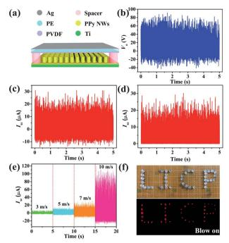
Fig. 5 (a) Device structure of the designed PPy NW-based W-TENG. (b)  $V_{\rm o}$ , (c)  $I_{\rm sc}$  and (d) the rectified  $I_{\rm sc}$  at a wind speed of 7 m s<sup>-1</sup> (on the scale of 4 BF). (e) The  $I_{\rm sc}$  at different wind speeds from 3 m s<sup>-1</sup> (2 BF) to 10 m s<sup>-1</sup> (5 BF). (f) Photographs of 40 LEDs before and after being powered by the W-TENG.
