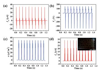
Fig. 3 (a) Short circuit current ( $I_{\rm sc}$ ), (b) output voltage ( $V_{\rm o}$ ), and (c) charge density ( $\sigma$ ) of the PPy NW-based TENG. (d)  $I_{\rm sc}$  of the PPy NW-based TENG in one direction after rectification. The inset is the photograph of 372 commercial LEDs powered by the PPy NW-based TENG.
