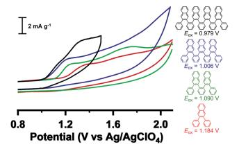
Fig. 4 Cyclic voltammetry of foldamers H-Ar-1 to H-Ar-4 in  $\rm CH_3CN$  containing 0.1 M  $\rm Bu_4NClO_4$  measured at 50 mV s $^{-1}$ .
