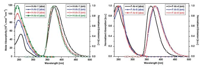
Fig. 3 UV-vis absorption and emission spectra ( $\lambda_{exc} = 260$  nm) of oligomeric series in CH<sub>2</sub>Cl<sub>2</sub>: (left) H-Ar-1 to H-Ar-4, (right) F-Ar-4 to F-Ar-6.
