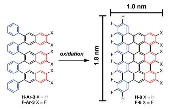
Scheme 3 o-Arylenes as precursors to nanographenes H-8 and F-8 with control of width and length dimensions in addition to potential control of edge-functionalization. Dimensions shown are estimated for H-8 based on DFT calculations and measurements between the furthest hydrogen atoms.
