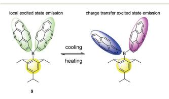
Fig. 9 Temperature-sensitive probe (9) based on emission mechanism change.
