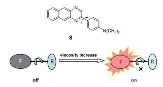
Fig. 8 Viscosity-sensitive fluorescence probe (8) and its response mechanism.
