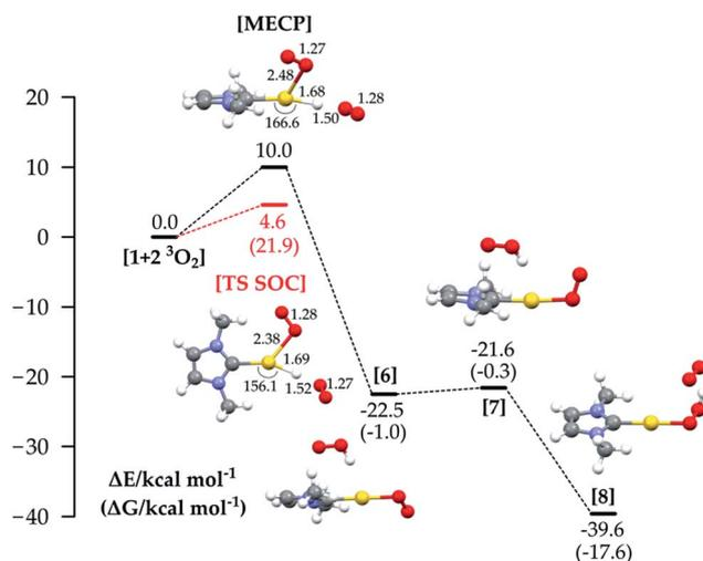
Fig. 5 Reaction energy profiles and structures for the mechanism involving two molecules of O<sub>2</sub> (the red line shows the energy of the TS optimized with SOC).  $\Delta G$  values are shown in brackets. All energy values (in kcal mol<sup>-1</sup>) refer to the energy of the isolated reactants (1 + <sup>3</sup>O<sub>2</sub> + <sup>3</sup>O<sub>2</sub>) taken as zero.
