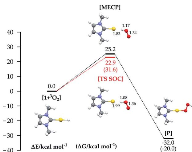
Fig. 3 Reaction energy profiles and structures for the hydrogen abstraction mechanism (the red line shows the energy of the TS optimized with SOC).  $\Delta G$  values are shown in brackets. All energy values (in kcal mol<sup>-1</sup>) refer to the energy of the isolated reactants taken as zero.
