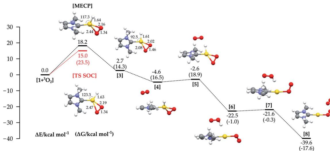
Fig. 4 Reaction energy profiles and structures for the oxidative addition/reductive elimination mechanism (the red line shows the energy of the TS optimized with SOC).  $\Delta G$  values are shown in brackets. All energy values (in kcal mol<sup>-1</sup>) refer to the energy of the isolated reactants taken as zero. For structures 4 to 8, the reactants are 1 + two isolated molecules of <sup>3</sup>O<sub>2</sub>.
