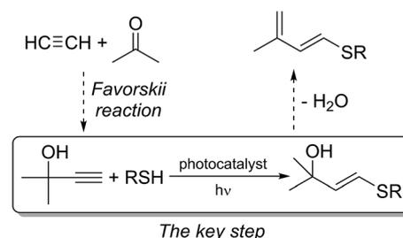
Scheme 1 The key light-mediated thiol–yne click reaction for the synthesis of activated dienes from simple precursors.
