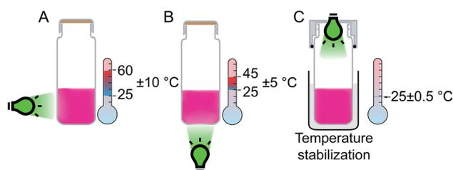
Fig. 1 Comparison of the possible designs of the photoreactor: (A) side irradiation (LED strip); (B) bottom irradiation (LED matrix); (C) developed design with temperature stabilization.
