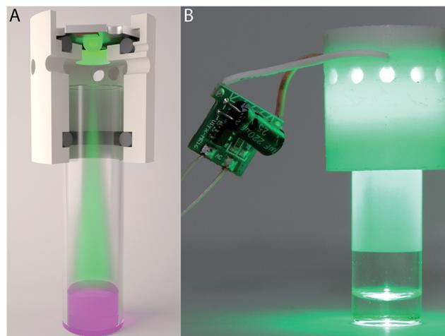
Fig. 2 Computer model of designed photoreactor (A) and ready to use assembled photoreactor (B).
