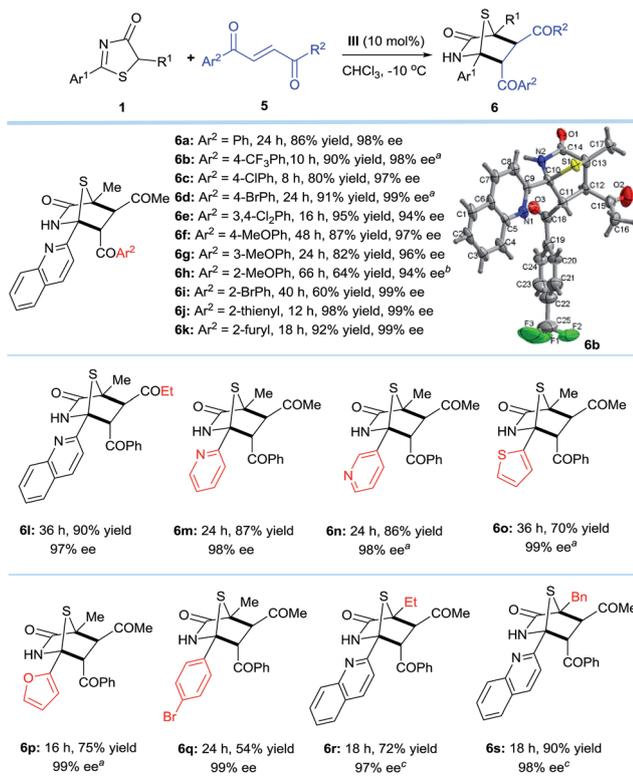
Scheme 3 Reaction conditions: **1** (0.2 mmol), **5** (0.3 mmol), **III** (0.02 mmol), CHCl<sub>3</sub> (4.0 mL) at -10 °C. All drs are >20 : 1. ees were determined via chiral phase high-performance liquid chromatography analysis. <sup>a</sup> T = -30 °C. <sup>b</sup> T = 20 °C. <sup>c</sup> T = 25 °C.
