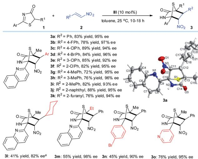
Scheme 1 Reaction conditions: **1** (0.2 mmol), **2** (0.4 mmol), **III** (0.02 mmol), toluene (4.0 mL) at 25 °C. All drs are >20 : 1. ees were determined *via* chiral HPLC analysis. <sup>a</sup> 72 hours.
