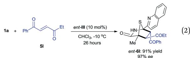
The reaction between 5H-thiazol-4-one **1a** and *trans*-4-oxo-4-phenylbutenone **5l** was conducted with 10 mol% of *D*-*tert*-leucine-based *ent*-**III** catalyst in chloroform at -10 °C (eqn (2)). The enantiomer of **6l** (*ent*-**6l**) was successfully obtained in 91% yield with 97% ee after 26 hours, thus demonstrating the potential of these dipeptide-based catalysts for enantiodivergent synthesis.
