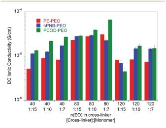
Fig. 3 lonic conductivity of unplasticized polymer electrolyte with different numbers of ethylene oxide (EO) units in the cross-linker and various [cross-linker] : [monomer] ratios at 25 °C. The data for PE–PEO SPEs are from ref. 10.
