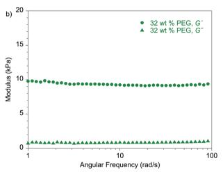
Fig. 7 Frequency-dependent dynamic shear measurements on (a) hPNB-PEO and (b) PCOD-PEO electrolytes. All membranes were plasticized with 32 wt% PEG 275 and had approximately 80 EO cross-linker units (88 for hPNB-PEO and 75 for PCOD-PEO), [1a]: [NB] or [1b]: [COD] ratios of 1:15, and [EO]: [Li] compositions of 20:1.
