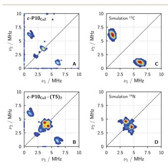
Fig. 5 Experimental HYSCORE spectra for  $c ext{-P10}_{Cu2}$  (A) and  $c ext{-}$  $P10_{Cu2} \cdot (T5)_2$  (B) recorded in regular toluene at 15 K and simulations of individual contributions to the experimental spectra using EasySpin for a  $^{13}$ C nucleus with hyperfine couplings of 4.0, 5.0 and 7.2 MHz for  $A_x$ ,  $A_{y}$ , and  $A_{z}$  (C) and a <sup>14</sup>N nucleus with hyperfine couplings of [-1.15] -1.14 -0.29] MHz and nuclear quadrupole couplings of [0.80 1.30 -2.101 MHz (D).
