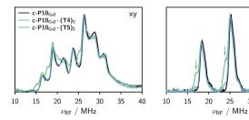
Fig. 4 Comparison of the  $^{14}$ N Davies ENDOR spectra of all three samples recorded at field positions corresponding to the xy (left) and z (right) orientations in frozen toluene- $d_8$  at 15 K. The green arrows indicate the additional nitrogen hyperfine coupling observed for c- $P10_{Cu2}$ ·( $T5)_2$ .
