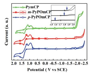
Fig. 3 Cyclic voltammograms of m-PyPOmCP and p-PyPOmCP and the reference compound PymCP measured in dilute CH<sub>2</sub>Cl<sub>2</sub> (anodic) and DMF (cathodic) solutions at a scan rate of 100 mV s<sup>-1</sup>. In the inserted figure, the blue arrows indicate the reduction onset of each compound.
