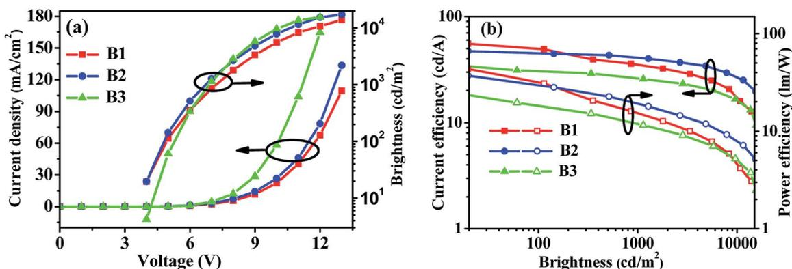
Fig. 6 (a) *J-V-L* characteristics and (b) efficiency curves for *m*-PyPomCP, *p*-PyPomCP and PymCP-hosted blue PhOLEDs B1, B2 and B3.
