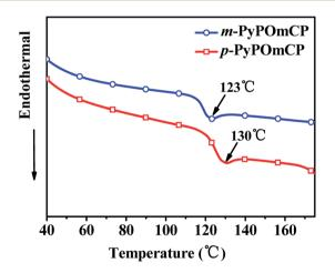
Fig. 1 DSC traces (at the second heating cycle) of m-PyPOmCP and p-PyPOmCP, recorded at a heating rate of 10  $^{\circ}$ C min $^{-1}$ .
