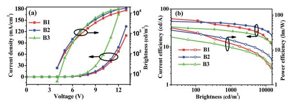
Fig. 6 (a) J-V-L characteristics and (b) efficiency curves for m-PyPOmCP, p-PyPOmCP and PymCP-hosted blue PhOLEDs B1, B2 and B3.
