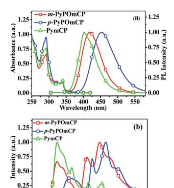
Fig. 2 (a) UV-vis absorption and PL spectra of m-PyPOmCP, p-PyPOmCP, and PymCP in dilute  $CH_2Cl_2$  solutions at 293 K. (b) LT PL spectra of m-PyPOmCP, p-PyPOmCP, and PymCP in a frozen 2-methyltetrahydrofuran matrix at 77 K.
