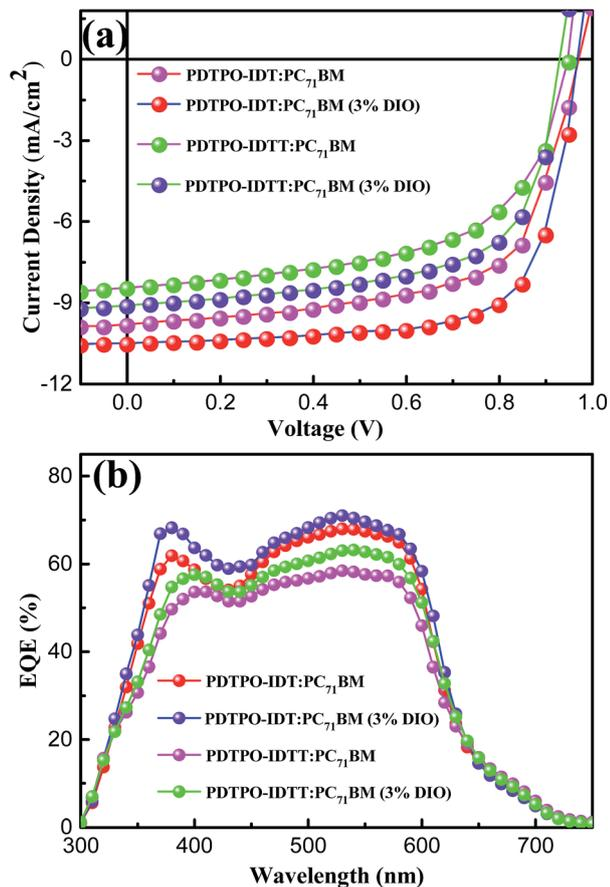
Fig. 4 (a)  $J$ - $V$  characteristics curves of PDTPO-IDT : PC<sub>71</sub>BM (1 : 2, w/w) and PDTPO-IDTT : PC<sub>71</sub>BM (1 : 2, w/w) based PSCs without or with 3% DIO (v/v) under AM 1.5 G at  $100 \text{ mW cm}^{-2}$ . (b) Corresponding EQE spectra of PDTPO-IDT : PC<sub>71</sub>BM and PDTPO-IDTT : PC<sub>71</sub>BM based PSCs without or with 3% DIO (v/v).
