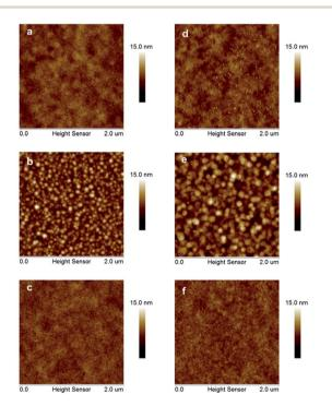
Fig. 6 AFM morphology images (2  $\mu$ m  $\times$  2  $\mu$ m). (a) PDTPO-IDT pure film, RMS: 0.88 nm. (b) PDTPO-IDT : PC<sub>71</sub>BM blend film without DIO, RMS: 1.62 nm. (c) PDTPO-IDT : PC<sub>71</sub>BM blend film with 3% DIO, RMS: 0.68 nm. (d) PDTPO-IDTT pure film, RMS: 0.99 nm. (e) PDTPO-IDTT : PC<sub>71</sub>BM blend film without DIO, RMS: 1.87 nm. (f) PDTPO-IDTT : PC<sub>71</sub>BM blend film with 3% DIO, RMS: 0.72 nm.
