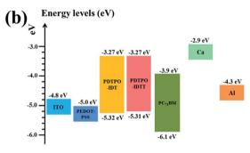
Fig. 2 (a) The electrochemical cyclic voltammetry measurements of PDTPO-IDT and PDTPO-IDTT thin film coated on the platinum electrode in acetonitrile solution containing  $0.1\,\mathrm{M}\,\mathrm{m}$ -Bu<sub>4</sub>NPF<sub>6</sub> at a scan rate of 100 mV s<sup>-1</sup>. (b) Schematic energy level diagram of all components used in conventional devices.
