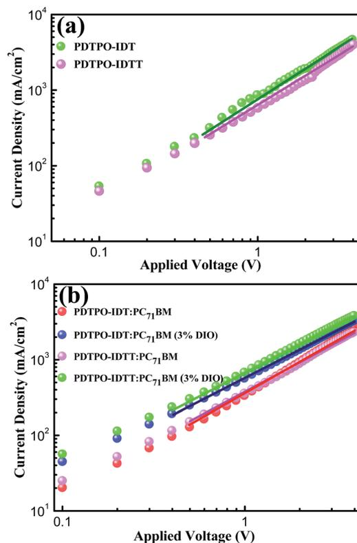
Fig. 5 Current-voltage ( $I$ - $V$ ) characteristics of pure films (a) and blend films (b) (with or without 3% DIO) PDTPO-IDT : PC<sub>71</sub>BM (1 : 2, w/w) and PDTPO-IDTT : PC<sub>71</sub>BM (1 : 2, w/w) in space-charge-limited current (SCLC) devices.
