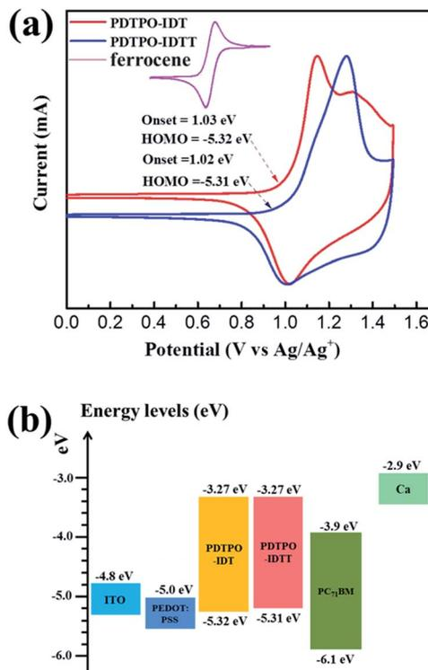
Fig. 2 (a) The electrochemical cyclic voltammetry measurements of PDTPO-IDT and PDTPO-IDTT thin film coated on the platinum electrode in acetonitrile solution containing  $0.1 \text{ M } n\text{-Bu}_4\text{NPF}_6$  at a scan rate of  $100 \text{ mV s}^{-1}$ . (b) Schematic energy level diagram of all components used in conventional devices.
