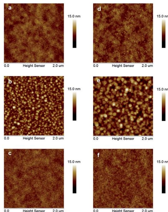
Fig. 6 AFM morphology images (2  $\mu\text{m} \times 2 \mu\text{m}$ ). (a) **PDTP0-IDT** pure film, RMS: 0.88 nm. (b) **PDTP0-IDT** : PC<sub>71</sub>BM blend film without DIO, RMS: 1.62 nm. (c) **PDTP0-IDT** : PC<sub>71</sub>BM blend film with 3% DIO, RMS: 0.68 nm. (d) **PDTP0-IDTT** pure film, RMS: 0.99 nm. (e) **PDTP0-IDTT** : PC<sub>71</sub>BM blend film without DIO, RMS: 1.87 nm. (f) **PDTP0-IDTT** : PC<sub>71</sub>BM blend film with 3% DIO, RMS: 0.72 nm.
