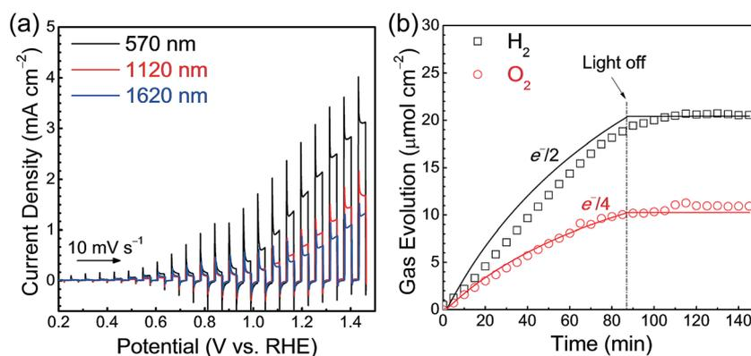
Fig. 4 (a) Current–potential curves obtained from Ta<sub>3</sub>N<sub>5</sub> photoanodes with different film thicknesses under simulated AM 1.5G light, and (b) time course of O<sub>2</sub> (open circles) and H<sub>2</sub> (open squares) gas evolution from a Ta<sub>3</sub>N<sub>5</sub>(570 nm)/Ta/Ti photoanode held at 1.23 V vs. RHE and a Pt counter electrode, respectively, under simulated AM 1.5G light. Solid curves represent the total charges estimated from the photocurrent.
