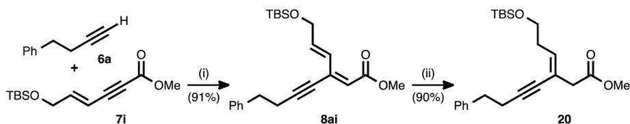
Scheme 3 Regio- and stereoselective reduction of a substrate featuring an extended  $\pi$ -system. Conditions: (i) 3 mol% Pd(OAc)<sub>2</sub>/TDMPP, 1.0 M in PhMe at 23 °C for 16 h. (ii) 5 mol% Cu(OAc)<sub>2</sub>·H<sub>2</sub>O/17, (EtO)<sub>2</sub>MeSiH (2 equiv.), *t*-BuOH (2 equiv.), 0.20 M in PhMe at 4 °C for 16 h.
