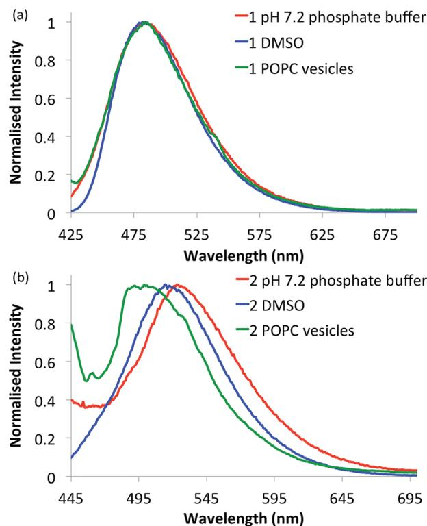
**Fig. 2** Normalised fluorescence emission spectra of selected naphthalimides. (a) Urea **1** (10 μM) and (b) thiourea **2** (10 μM) in various environments: 0.5% DMSO in pH 7.2 aqueous phosphate buffer (5 mM phosphate salts) (red curves), DMSO alone (blue curves) and in 1-palmitoyl-2-oleoyl-*sn*-glycero-3-phosphocholine (POPC) lipid vesicles (1 mM suspended in phosphate buffer) (green curves). See ESI<sup>†</sup> for respective emission spectra of all compounds.
