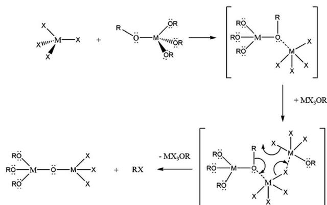
**Scheme 1** Non-hydrolytic condensation of metal halide and metal alkoxide to form an alkoxo-bridge intermediate. A "catalyst",  $\text{MX}_3\text{OR}$ , initiates conversion of the alkoxo-bridge to an oxo-bridge then subsequently eliminates an alkyl halide to form the desired metal oxide-product.
